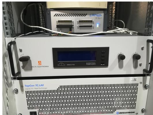
Figure 12.1.4: Delta Elektronika AD/DC power supply.
