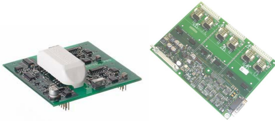
Figura 3 - IGBT Driver Core (a sinistra) e Driver Board (a destra).
