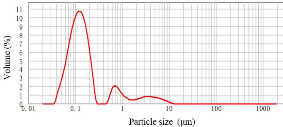
*Figure 10.11 : Particle size distribution of  $\text{Al}_2\text{O}_3$  powders. [15]*
