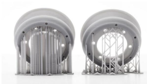
*Figure 3.4 : SLA part with supports (polymer)*
