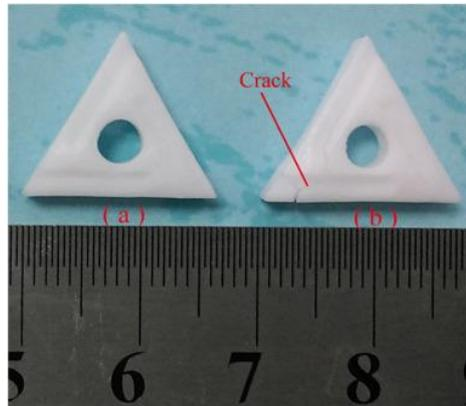
*Figure 8.5 : Sintered body obtained from (a) a two-step profile debinding; (b) vacuum debinding. [18]*
