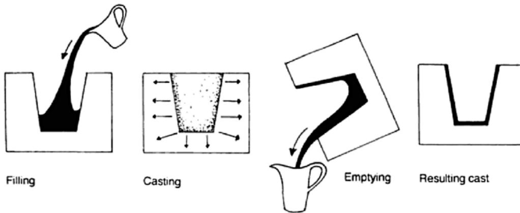
Figure 2.3 : Slip casting [29]
