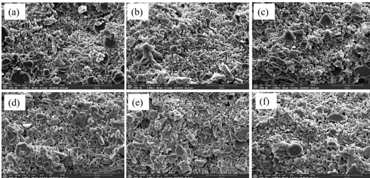
*Figure 8.12 : SEM of sintered samples (5000×): (a) 1100°C; (b) 1150°C; (c) 1200°C; (d) 1250°C; (e) 1300°C; (f) 1350°C. [15]*
