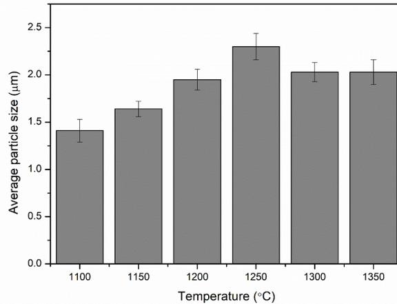
Figure 8.13 : Particle size of the samples after sintered at different temperatures [15]
