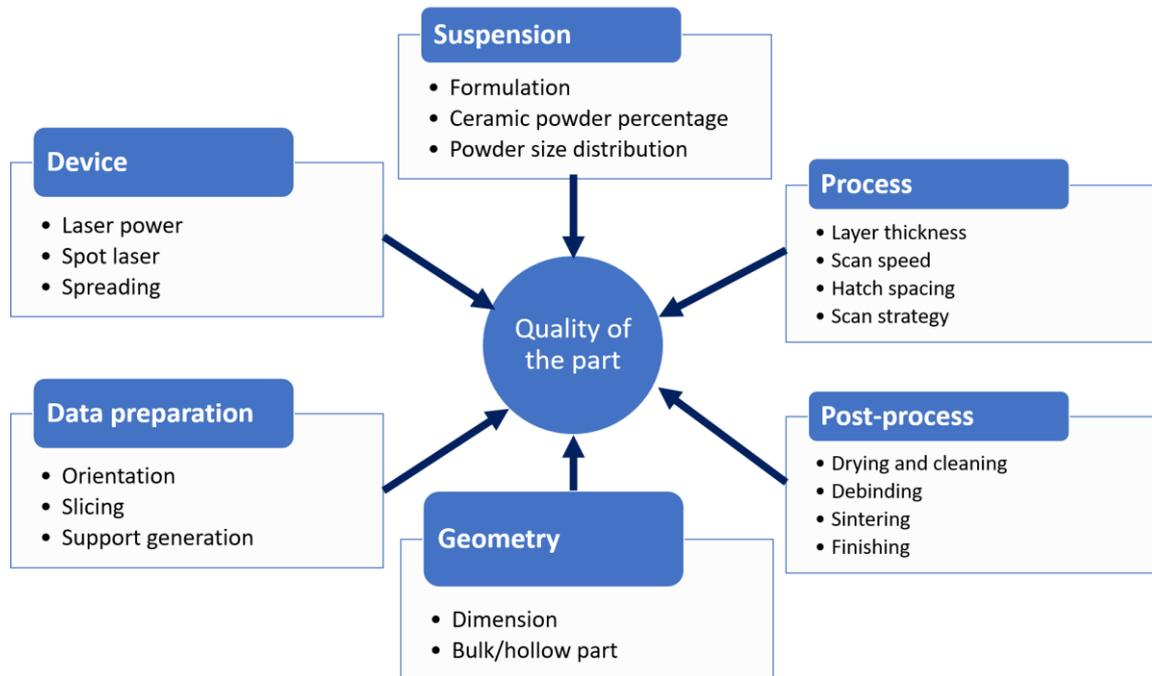
*Figure 1 : Parameters influencing quality of a part in SLA*
