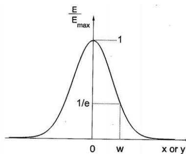
Figure 4.3: Gaussian intensity profile [39]
