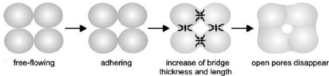
*Figure 5.1 : Different phase of sintering process [46]*
