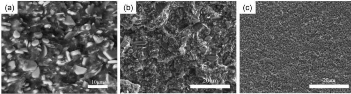
Figure 6.1 : SEM images of the green bodies (a) sample 1, (b) sample 2, (c) sample 3. [13]
