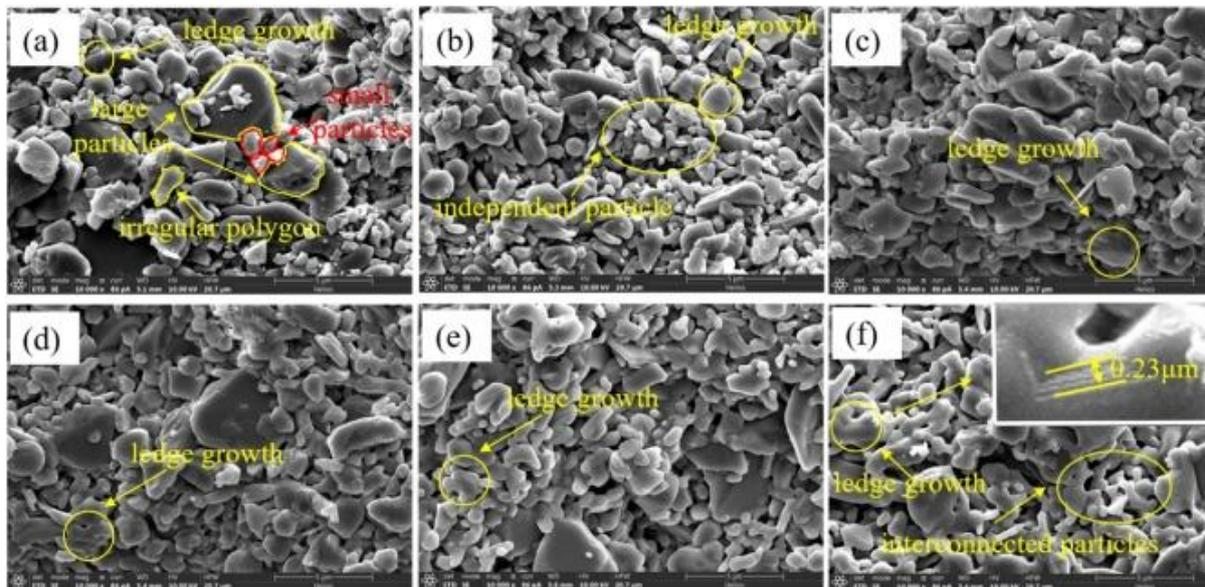
Figure 8.14 : SEM images (10,000× magnification) of samples sintered at (a) 1100, (b) 1150, (c) 1200, (d) 1250, (e) 1300, and (f) 1350 °C. [15]
