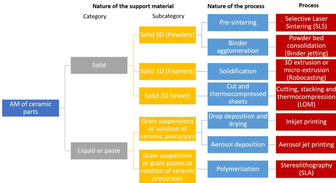
Figure 3.8 : Classification of AM techniques for ceramics
