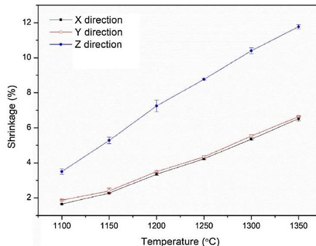
*Figure 8.15 : Shrinkage in samples sintered at different temperatures in vacuum [15]*
