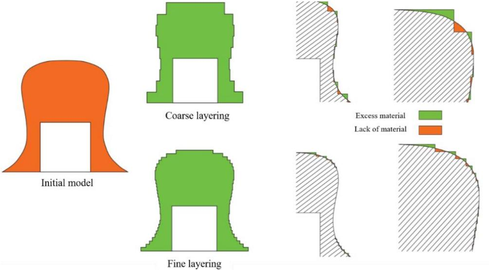
Figure 3.5 : Illustration of how a part is obtained by stacking layers [6]
