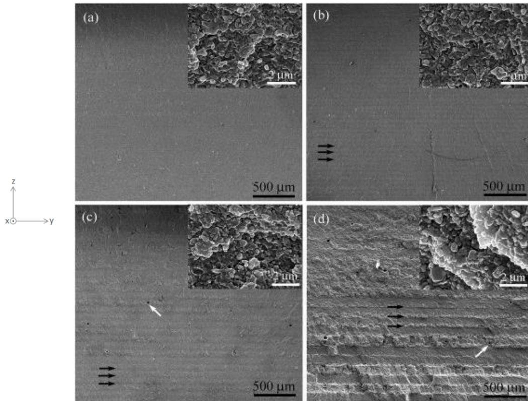
Figure 7.6 : Micrographs of green bodies with different layer thickness: (a) 30; (b) 60; (c) 90; (d) 120  $\mu\text{m}$ . [16]
