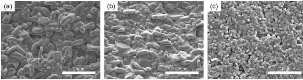
Figure 8.7 : SEM images revealing the morphology of the samples subjected to the **vacuum debinding** process: (a) sample 1, (b) sample 2, (c) sample 3. [13]
