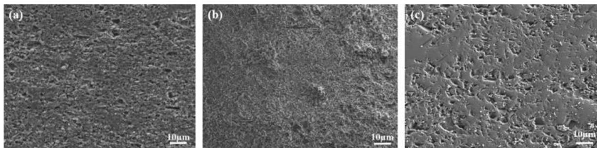
*Figure 8.1: SEM images of 3D printed alumina samples (a) as-printed (b) after debinding and (c) after sintering [17]*
