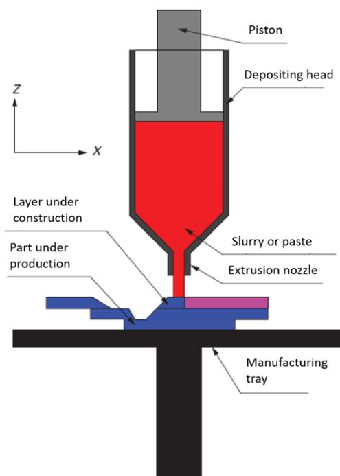
Figure 3.11 : Robocasting process [6]
