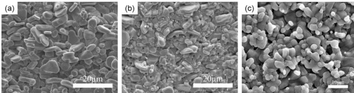
Figure 6.2 : SEM images revealing the morphology of the samples subjected to the thermal debinding process: (a) sample 1, (b) sample 2, (c) sample 3. [13]
