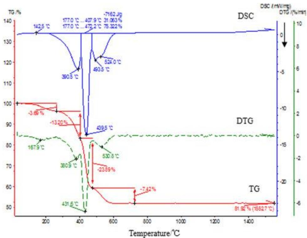
Figure 10.10 : Thermal decomposition behavior of the green bodies. (The DTG curve is the derivative of the TGA curve.).
