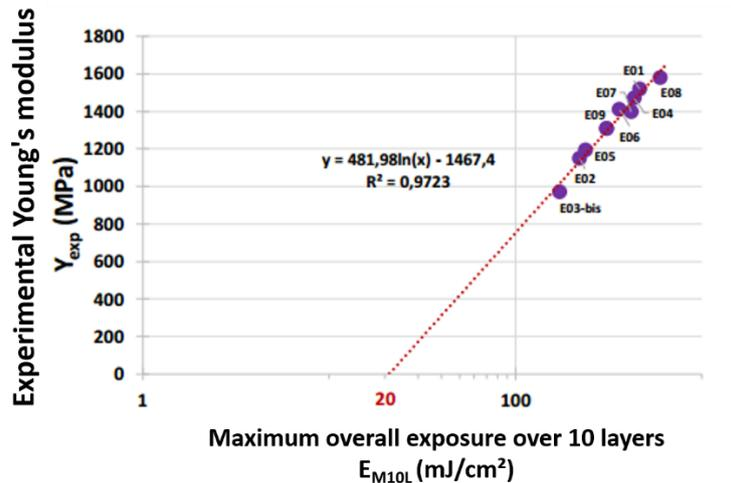
Figure 7.2 : Young's modulus as a function of E10L for green alumina parts [8]
