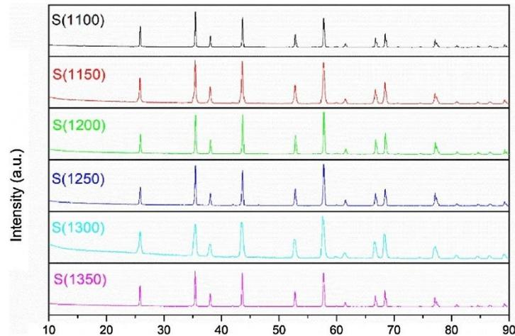
*Figure 10.8 : XRD patterns from samples sintered at different temperatures in vacuum [15]*
