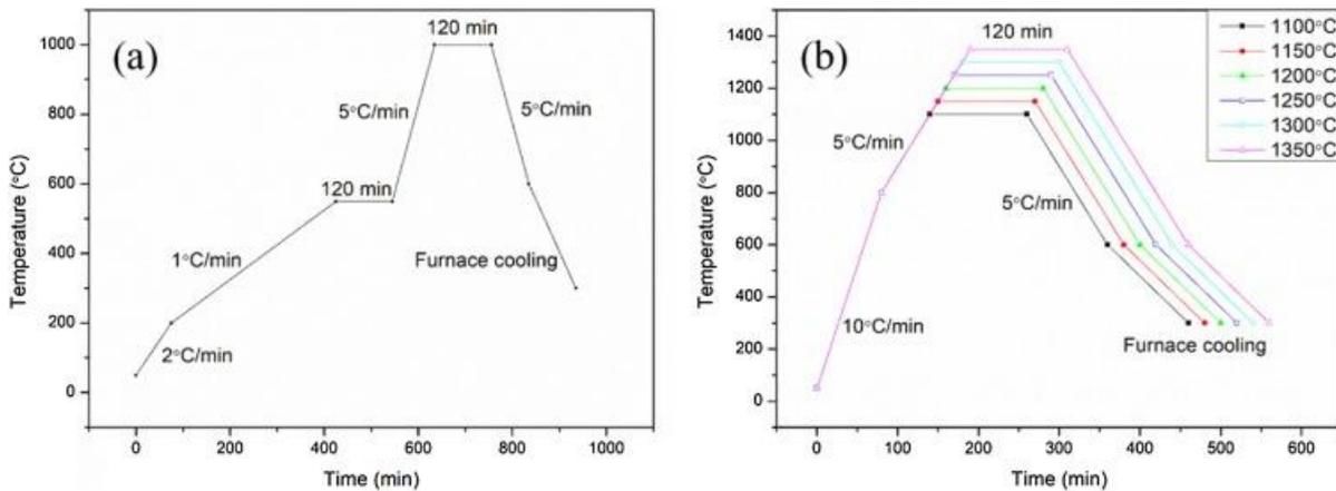
*Figure 10.12 : Thermal cycles of green bodies: (a) debinding; (b) sintering [15]*
