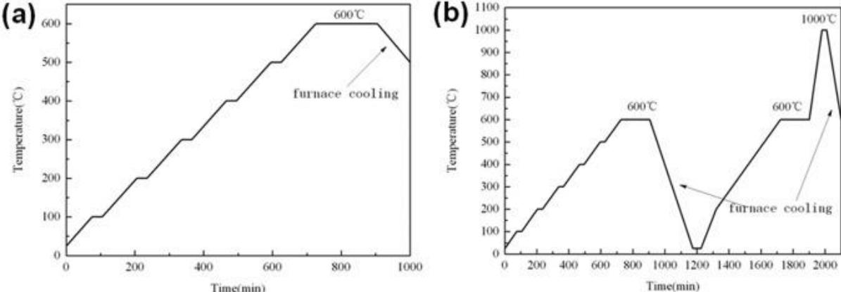
Figure 8.3 : (a) The air pyrolysis debinding and the vacuum debinding profile and (b) the two-step debinding profile. [18]
