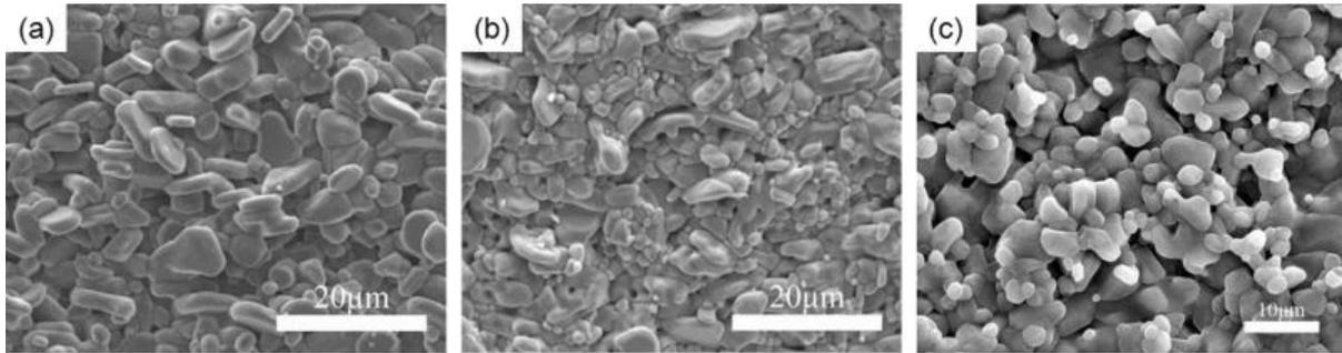
Figure 8.8 : SEM images revealing the morphology of the samples subjected to the **thermal debinding** process: (a) sample 1, (b) sample 2, (c) sample 3. [13]
