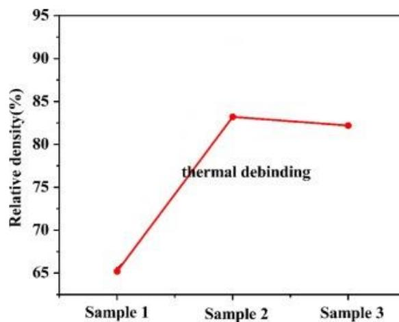
Figure 6.3 : Densities of the different samples after thermal debinding. [13]
