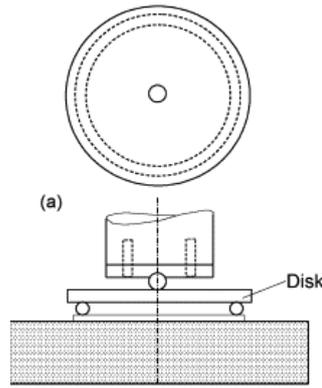
Figure 10.2: Diagram of the biaxial ball-on-ring method [55]
