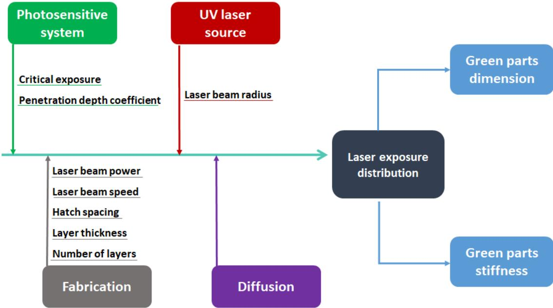
Figure 7.1 : Diagram of factors influencing the SLA process [8]
