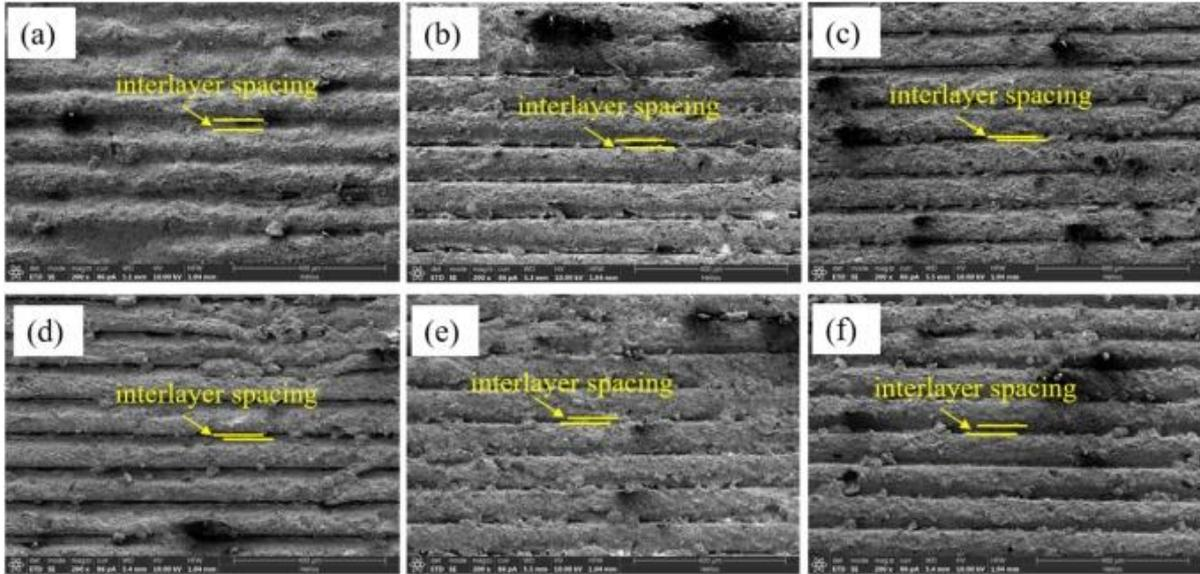
Figure 8.10 : SEM images showing delamination during sintering at (a) 1100, (b) 1150, (c) 1200, (d) 1250, (e) 1300, and (f) 1350 °C. [15]
