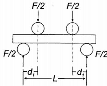
Figure 10.3 : Diagram of the four-point bending test [56]
