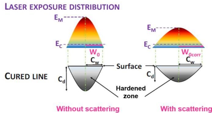
Figure 4.6 : Impact of the scattering phenomenon on the distribution of the laser beam exposure and the hardened line [11]
