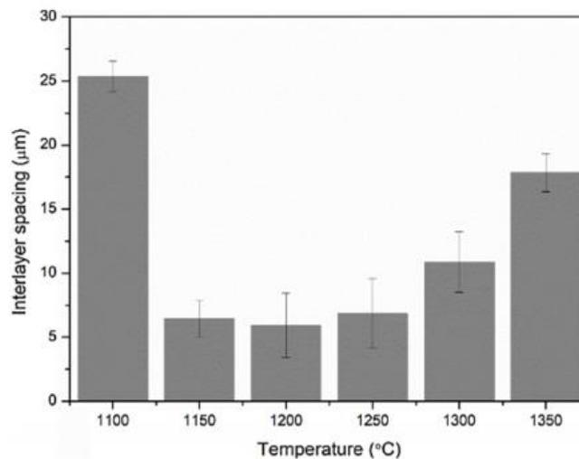
Figure 8.11 : Variation of interlayer spacing according to sintering temperature [15]
