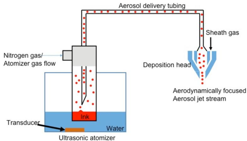
*Figure 3.14 : Aerosol printing process [37]*
