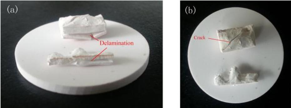
Figure 8.4 : Defects for samples debound in air (a) delamination (b) cracks
