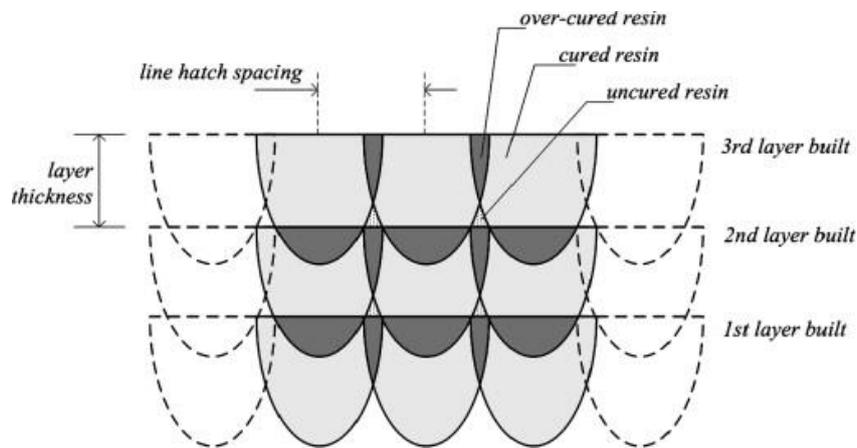
*Figure 4.7 : Microstructure section of parts showing three constructed layers [42]*
