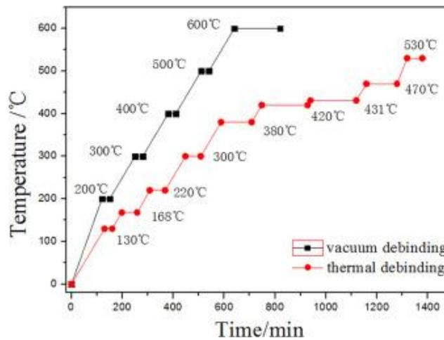
Figure 8.6 : Temperature curves used for the debinding of the Al<sub>2</sub>O<sub>3</sub> ceramics prepared through SLA [13]
