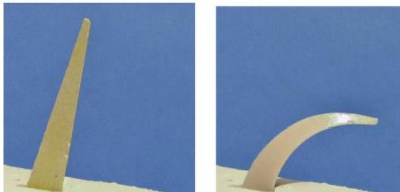
*Figure 1.1 : Temperature measurement using fuse watches [20]*
