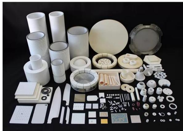
Figure 1.3 : Diversity of components in alumina
