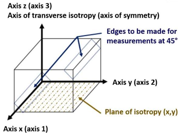
Figure 7.3 : Definition of measurement axes [51]
