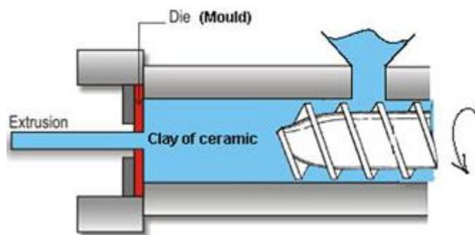
Figure 2.4 : Extrusion process [30]
