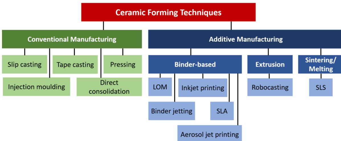
Figure 2.2 : Shaping for ceramics
