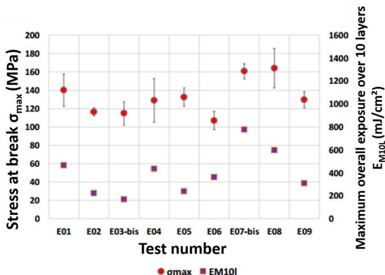
Figure 7.5 : Stress at break and exposure according to experiments (E03-bis = E03 and E07-bis = E07) [8]
