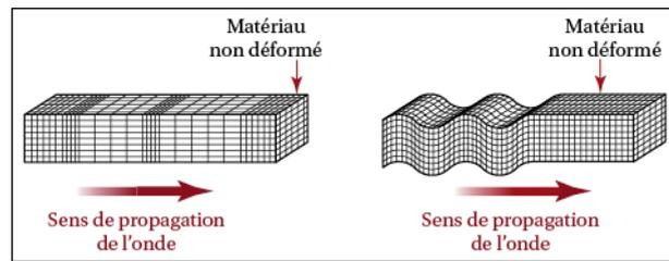
Figure 10.1 : Diagram of a longitudinal (left) and transverse (right) wave [54]
