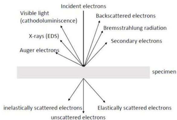
Figure 10.6 : Electron interaction with matter [60]
