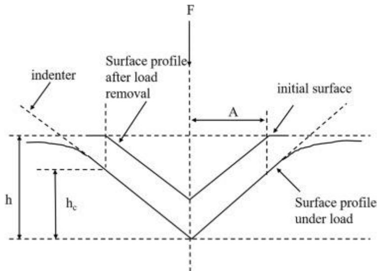
Figure 10.4 : Nanoindentation schematic. [59]
