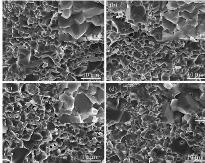
Figure 7.7 : SEM micrographs for the cross-sectional surfaces of sintered alumina with different layer thickness (a) LT30; (b)LT 60; (c) LT90; (d) LT120. [16]
