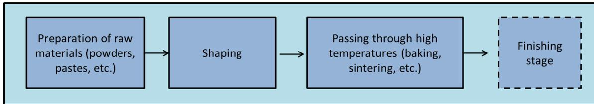
Figure 2.1 : Steps in the elaboration of a ceramic piece
