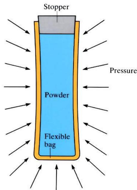
*Figure 2.5 : Cold isostatic pressing [31]*
