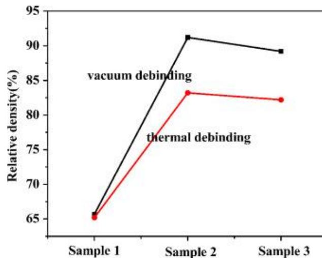
Figure 8.9 : Comparison of the relative densities of the different samples after the vacuum and thermal debinding. [13]
