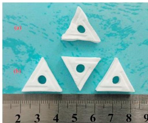
Figure 8.2 : (a) The green body dried via a natural drying process and (b) the green body dried via a liquid desiccant (PEG)-assisted drying process. [18]
