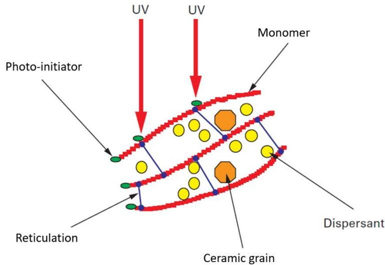
Figure 4.2 : Constituents of a reactive suspension [6]
