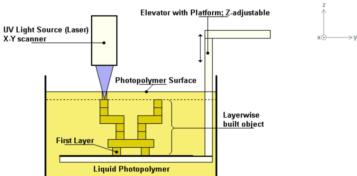
Figure 4.1 : Stereolithography process [38]
