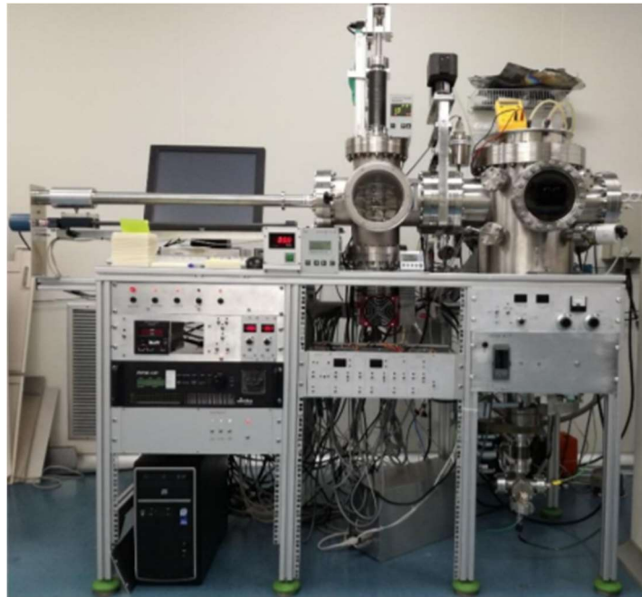
Figure 16: The ultra-high vacuum sputtering system used in this work.
