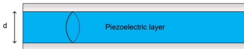
Figure 4: Standing wave formation in a BAW resonator.
