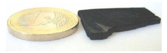
Figure 3 - Photos of the "carpet" of carbon nanotubes
