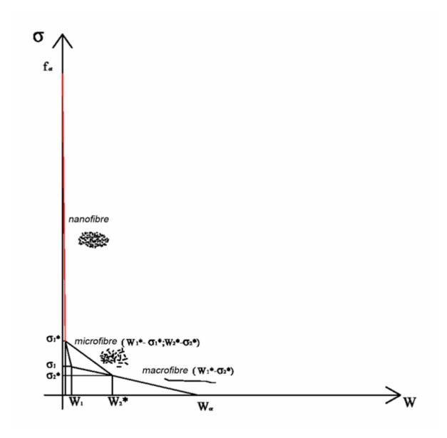
Figure 2 - Hypothetical fibermetric curve
