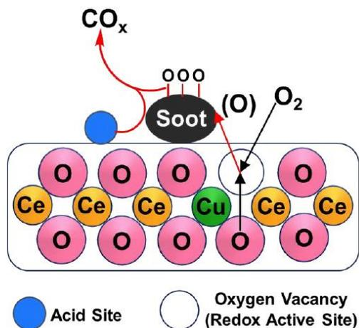
**Figure 9.7:** Role of acid sites in the soot oxidation reaction on ceria catalysts from ref. [101]
