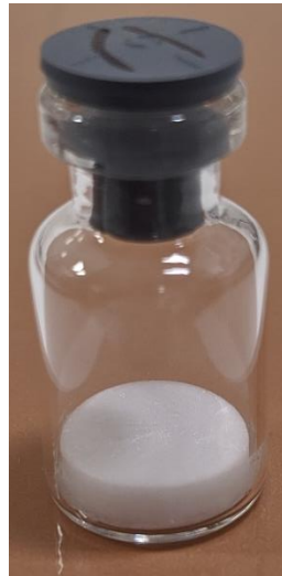
Figure 3.27: Product obtained after freeze drying by a siliconized vial filled with 5% w/w sucrose + 0,02% w/v Tween 80 that underwent the degassing procedure before the freezing one.
