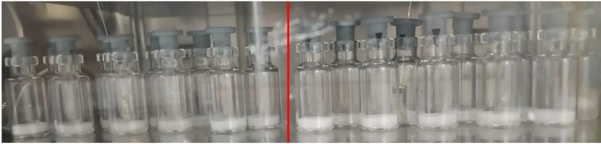
Figure 3.19: Two group of TopLyo® vials filled with with demineralized water + 0,02% w/v Tween 80 at the end of the nucleation process. The group of samples on the left was subject to degassing, while the group on the right was not.
