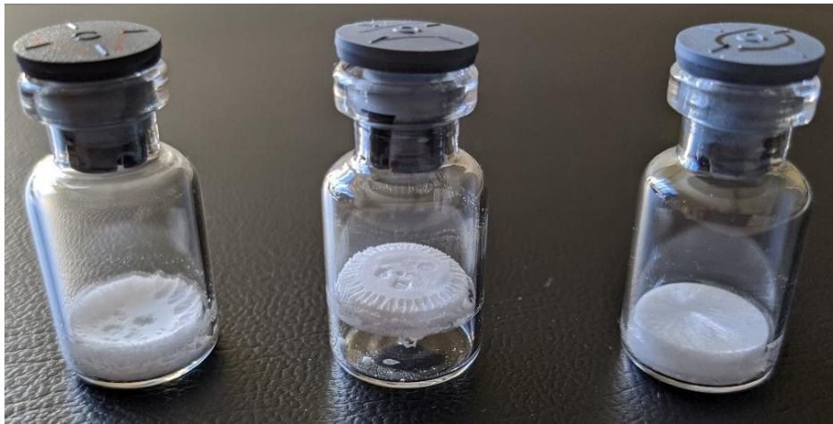
Figure 4.1: From the left to the right the image shows the product obtained after freeze drying of 5% w/w sucrose in untreated vials, 5% w/w sucrose in siliconized vials and degassed 5% w/w sucrose + 0,02% w/v Tween 80 in siliconized vials.
