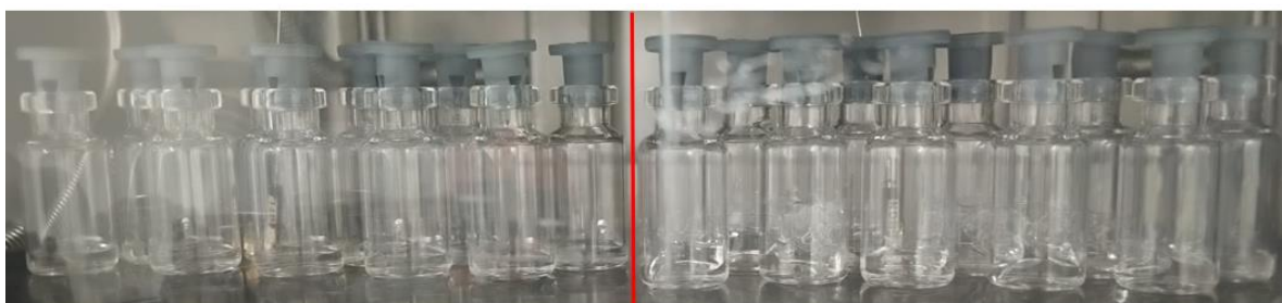
Figure 3.22: Two group of TopLyo® vials filled with 5% w/w mannitol + 0,02% w/v Tween 80. The group of samples on the left was subject to degassing, while the group on the right was not. In the group on the right could be observed bubbling phenomenon due to the decrease in pressure in the vacuum chamber.
