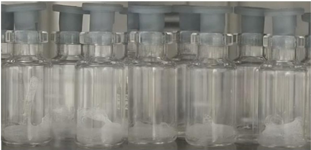
Figure 3.6: Irregular cake in TopLyo ® vials filled with demineralized water; the nucleation occurred because of the boiling.
