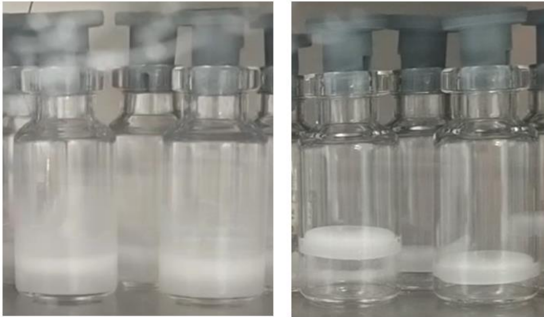
Figure 3.9: On the left there are sulphate treated vials, while on the right TopLyco® vials both filled with 5% w/w mannitol; the vials were just nucleated.
