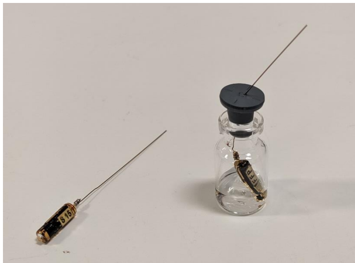
Figure 2.5: Tempris probe on the left and Tempris probe correctly inserted in a vial on the right.
