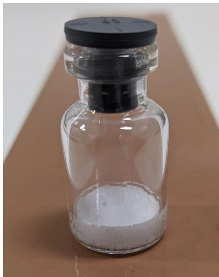
Figure 3.23: Product obtained after freeze drying by an untreated vial filled with 5% w/w sucrose.
