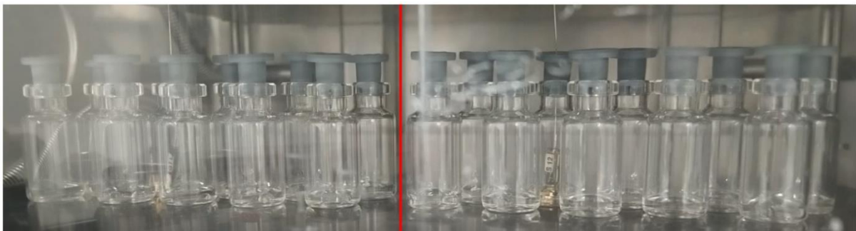
Figure 3.16: Two group of TopLyo® vials filled with demineralized water. The group of samples on the left was subject to degassing, while the group on the right was not. In both could be observed boiling phenomenon due to the decrease in pressure in the vacuum chamber.
