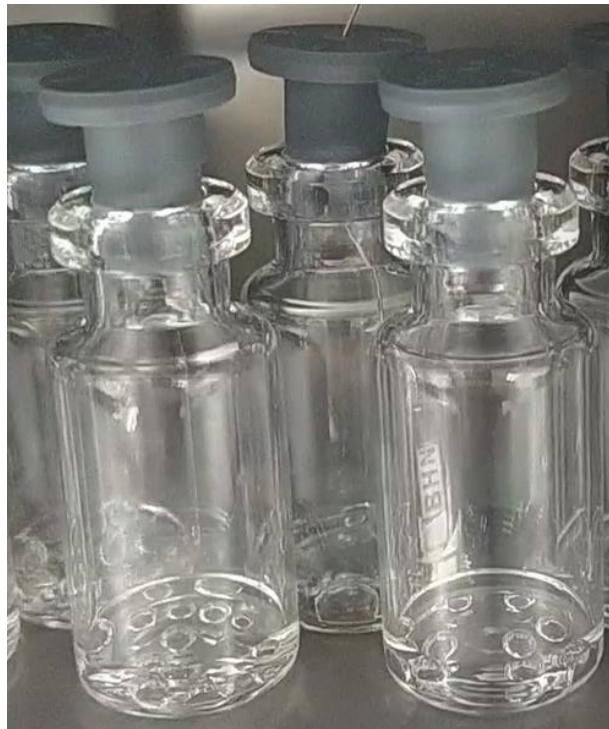
Figure 3.4: Small bubble in TopLyo ® vial filled with 5% w/w sucrose+ 0,02% w/v Tween 80 with a pressure exerted on the liquid of 20 mbar.
