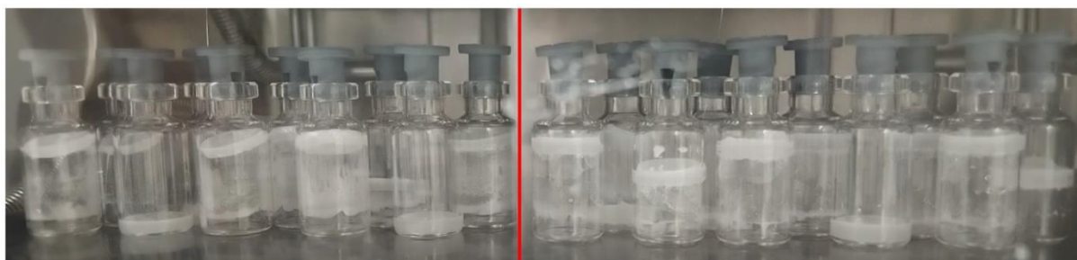
Figure 3.21: Two group of TopLyo® vials filled with with 5% w/w sucrose + 0,02% w/v Tween 80 at the end of the nuclation process. The group of samples on the left was subject to degassing, while the group on the right was not.
