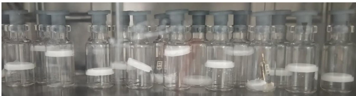
Figure 3.13: TopLyo® vials filled with 5% w/w mannitol at the end of the Experiment 2.
