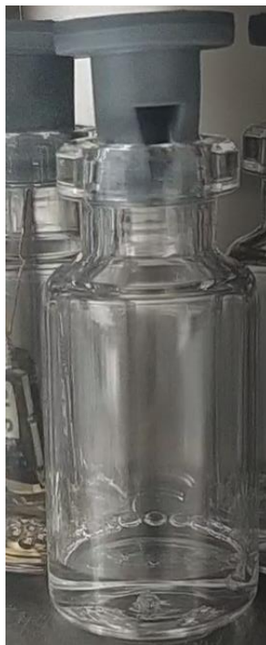
Figure 3.2: Small bubble in TopLy o ® vial filled with Demineralized water + 0,02% w/v Tween 80 with a pressure exerted on the liquid of 30 mbar.
