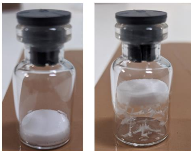
Figure 3.26: Product obtained after freeze drying by a siliconized vial filled with 5% w/w sucrose + 0,02% w/v Tween 80. On the left there is a vial in which the blow up is almost absent, while on the right one in which it is present.
