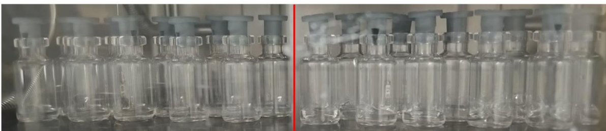
Figure 3.20: Two group of TopLyo® vials filled with 5% w/w sucrose + 0,02% w/v Tween 80. The group of samples on the left was subject to degassing, while the group on the right was not. In the group on the right could be observed bubbling phenomenon due to the decrease in pressure in the vacuum chamber.
