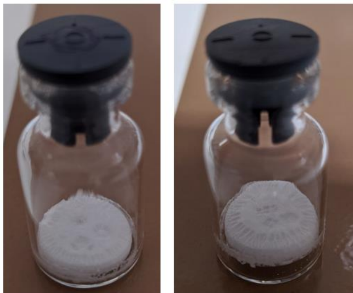
Figure 3.24: Product obtained after freeze drying by a siliconized vial filled with 5% w/w sucrose. On the left there is a vial in which the blow up is absent, while on the right one in which it is present.
