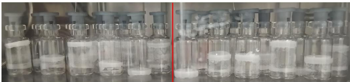
Figure 3.23: Two group of TopLyo® vials filled with with 5% w/w mannitol + 0,02% w/v Tween 80 at the end of the nucleation process. The group of samples on the left was subject to degassing, while the group on the right was not.
