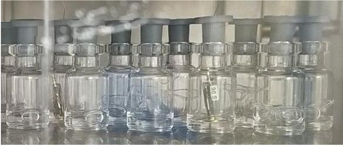
Figure 3.3: Bubble going up and bursting into untreated vial filled with 5% w/w mannitol+ 0,02% w/v Tween 80 with a pressure exerted on the liquid of 6 mbar.
