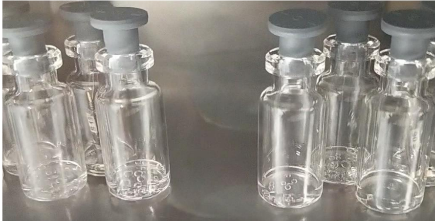
Figure 3.15: Two group of TopLyo® vials filled on the left with demineralized water, while on the right with water for injection. Decreasing the pressure both the solutions formed bubbles on the bottom of the container, as typical of the boiling phenomenon.
