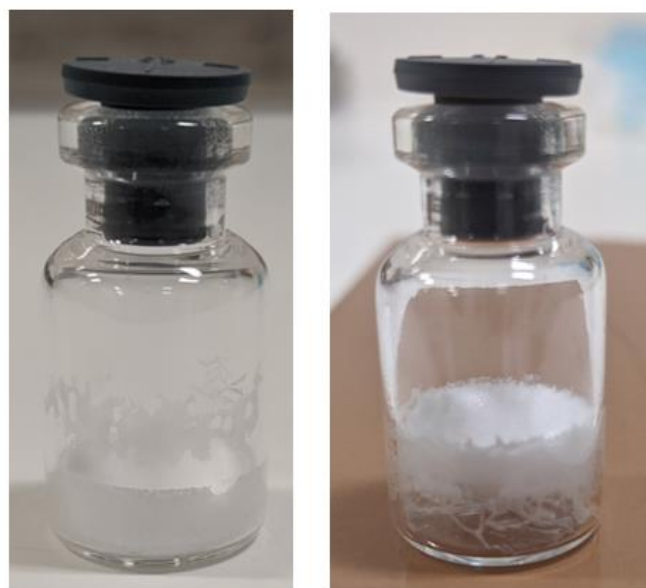
Figure 3.25: Products obtained after freeze drying by an untreated vial filled with 5% w/w sucrose + 0,02% w/v Tween 80. On the left there is a vial in which the blow up is absent, while on the right one in which it is present.
