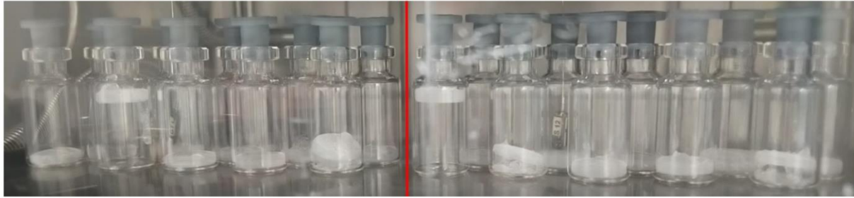
Figure 3.17: Two group of TopLyo® vials filled with demineralized water at the end of the nucleation process. The group of samples on the left was subject to degassing, while the group on the right was not.
