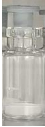
Figure 3.7: Regular cake in TopLyo® vials filled with demineralized water; the nucleation didn't occur because of the boiling.
