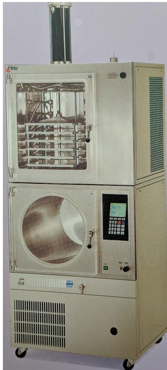
Figure 2.4: pilot-scale freeze-dryer HETO DW 8030. Figure taken from Heto-Holten Lab Equipment brochure with modifications.
