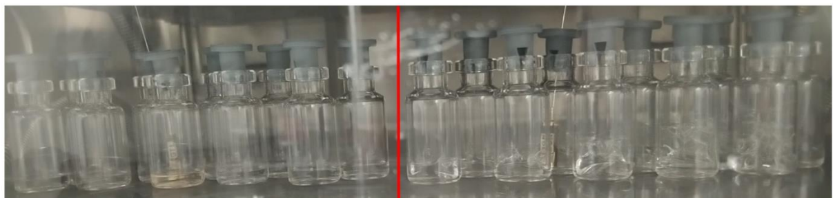
Figure 3.18: Two group of TopLyo® vials filled with demineralized water + 0,02% w/v Tween 80. The group of samples on the left was subject to degassing, while the group on the right was not. In the group on the right could be observed bubbling phenomenon due to the decrease in pressure in the vacuum chamber.
