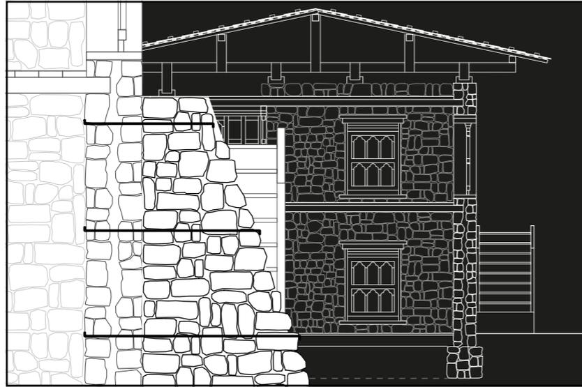
New stone walls are constructed in order to counteracting horizontal loads. New walls are located in one or both directions. A different solution is the construction of buttresses. Another one is increasing the wall thickness, increasing the resisting area.
