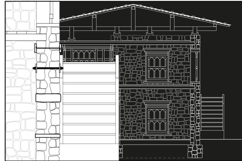
Transversal bonding elements are placed inside the walls to improve shear behaviour. This strategy imposes the creation of a hole in the wall, removing stones without disturbing the others, and the consequent filling of that with concrete or anti-shrinkage mortar.
