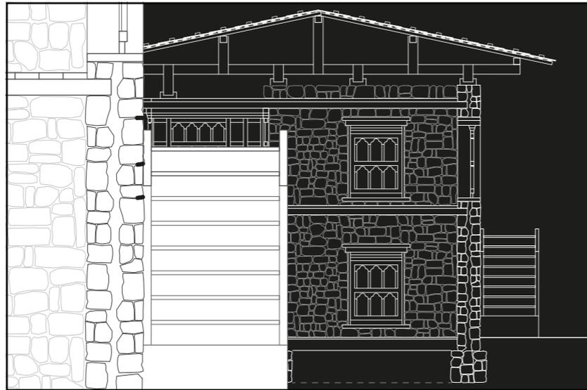
Deep re-pointing is applied in order to prevent damages caused by weakening over time. A re-pointing is a simple one when the mortar joints is partially replaced with better quality mortar. This action is called reinforced deep re-pointing when the replacement is preceded by the insertion of reinforced rods or strips inside the joints.
