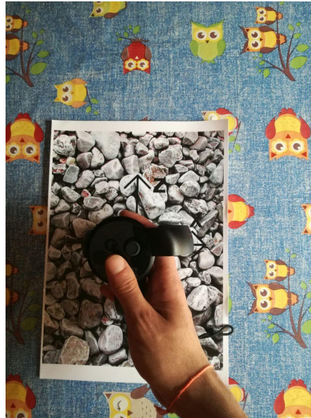
Figure 1.2: Figure of how the headset controller should be positioned on the landmark to coordinate VR world with AR World
