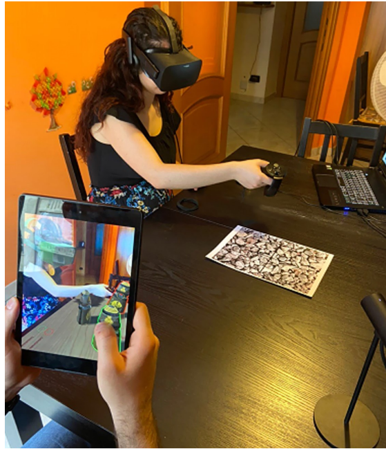
Figure 4.1: Figure showing how the VR user sees the other one manipulating an object, which perfectly overlaps in the two worlds
