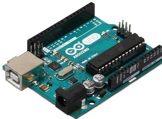
Figure 4.2: Arduino Uno board
