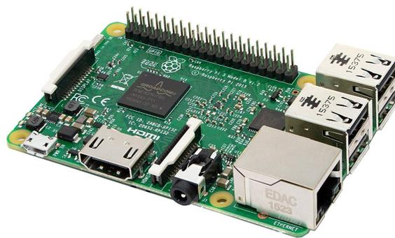
Figure 4.1: Raspberry 3 model B board
