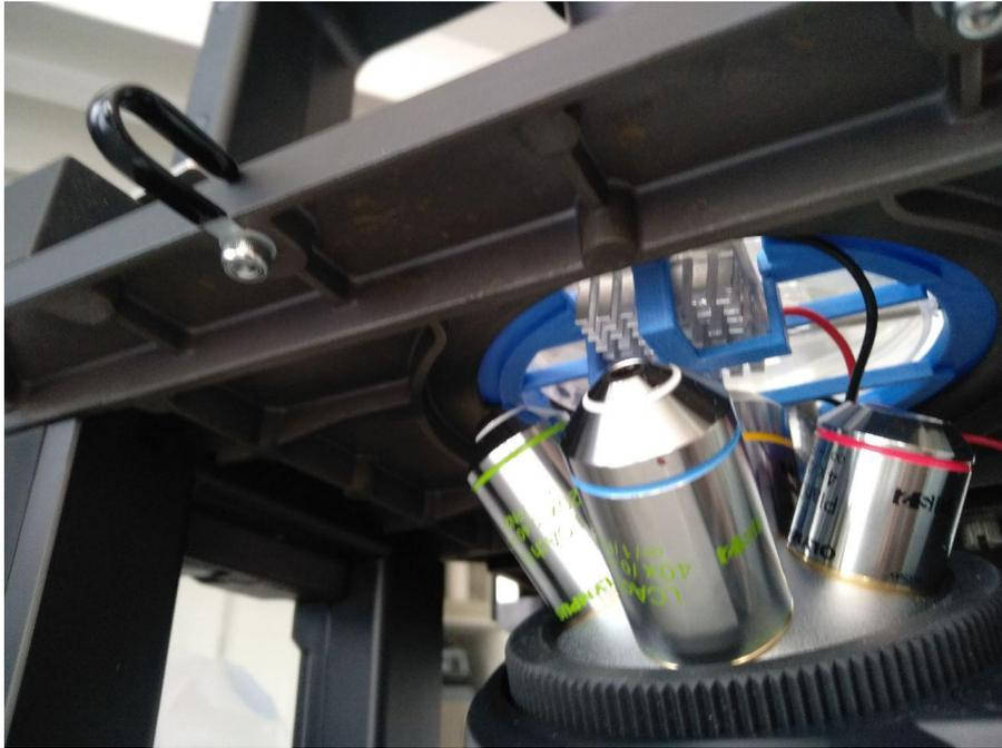
Figure 6.7: View from the bottom of the *Heating chamber* on the inverted microscope: the lenses have enough space to rotate without touching the structure
