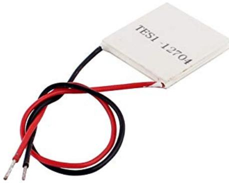
Figure 4.5: The Peltier cell *TES1*
