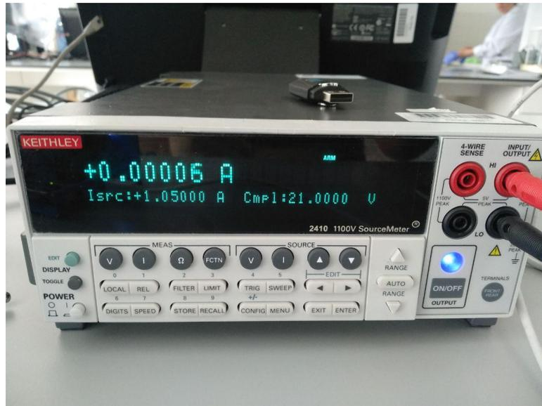
Figure 4.4: The power supply *Keithley 2410*
