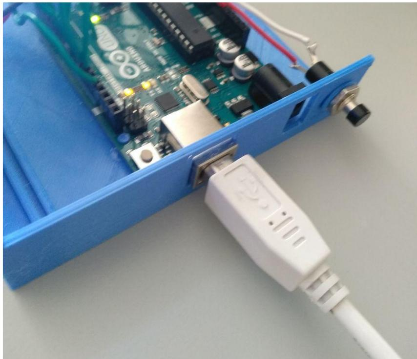
Figure 6.14: Close-up on the left side of the *Case*: the apertures for the power and USB cables of Arduino, as well as the black pushbutton, are visible.
