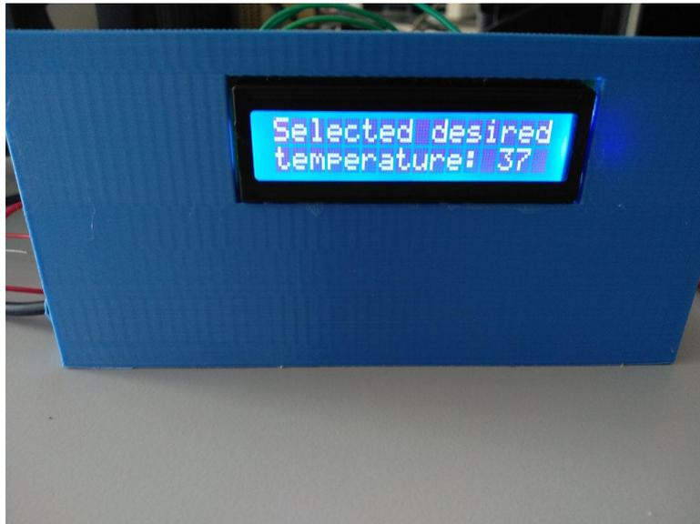
Figure 5.2: Desired temperature selected
