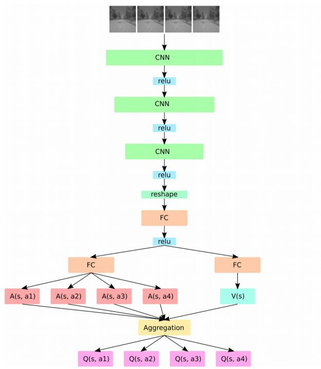
*Figure 4.9 Autonomous Emergency Steering Neural Network*
