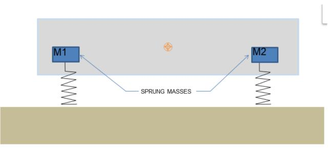
Figure 3.4 Vehicle representation as a collection of sprung masses of mass M1 and M2 [33]
