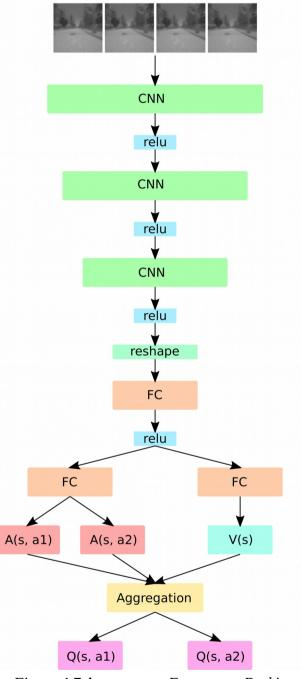
Figure 4.7 Autonomous Emergency Braking Neural Network
