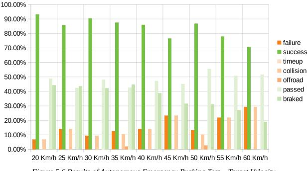
Figure 5.6 Results of Autonomous Emergency Braking Test – Target Velocity
