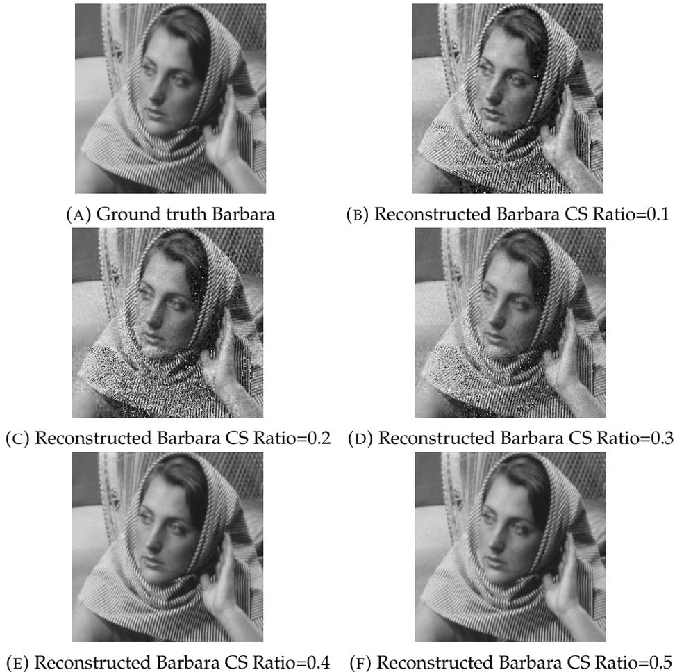
FIGURE 5.6: Reconstructed image for block size = 32 and CS Ratio=0.1-0.5
