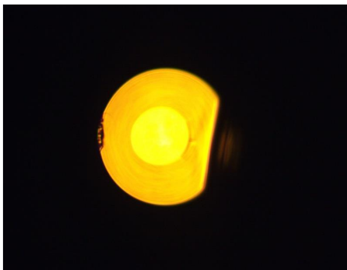
Figure 2.9: Fiber Cross Section at the optical Microscope
