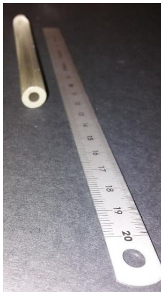
Figure2.4: Final Preform picture after all polishing procedure
