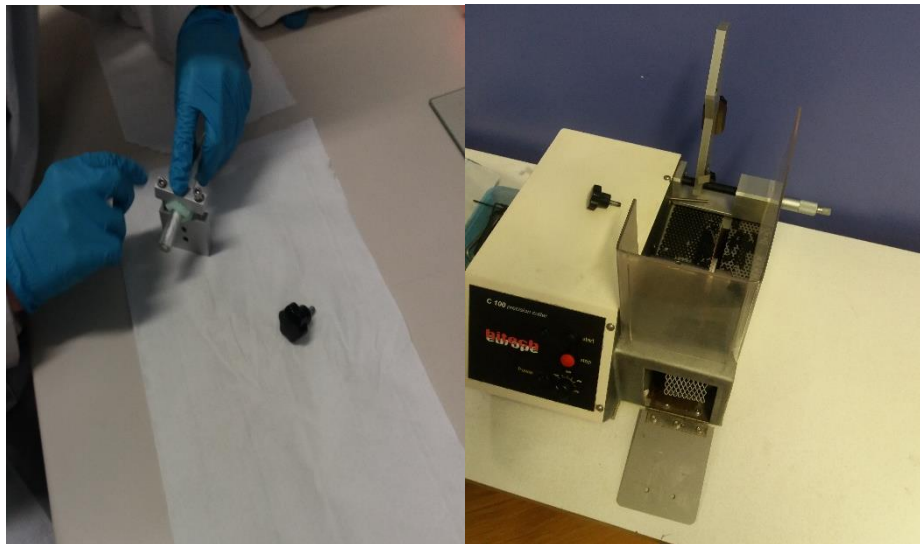
Figure2.1: Left: The instrument which will clamp the preform for cutting the sample on it. Right: ceaser cutter Machine
