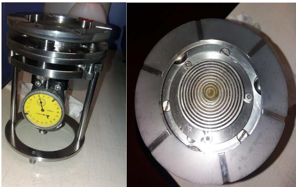
Figure 2.3 Left: Geake Equipment from body side of view Right: Polished Sample of Optical cladding preform
