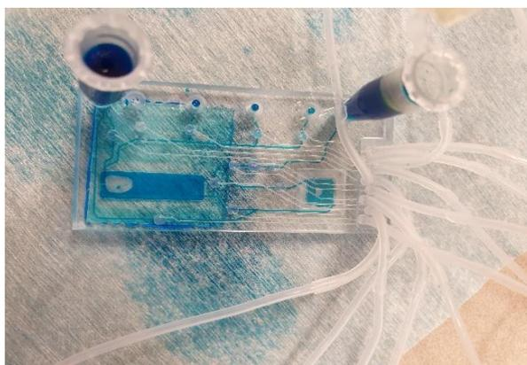
*Figure 55. Unsuccessful priming attempt, with internal bubbles still present*
