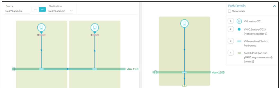
Figure 5.4- network topology flow path between web server source and database destination
