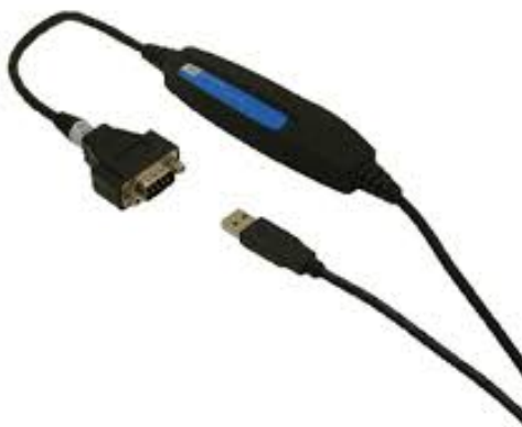
Figure 3.3: Kvaser leaflight device. Taken from [38]
