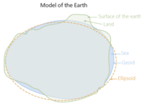
Figure 4.2: Mean sea level is approximated by geoid. Taken from [51]
