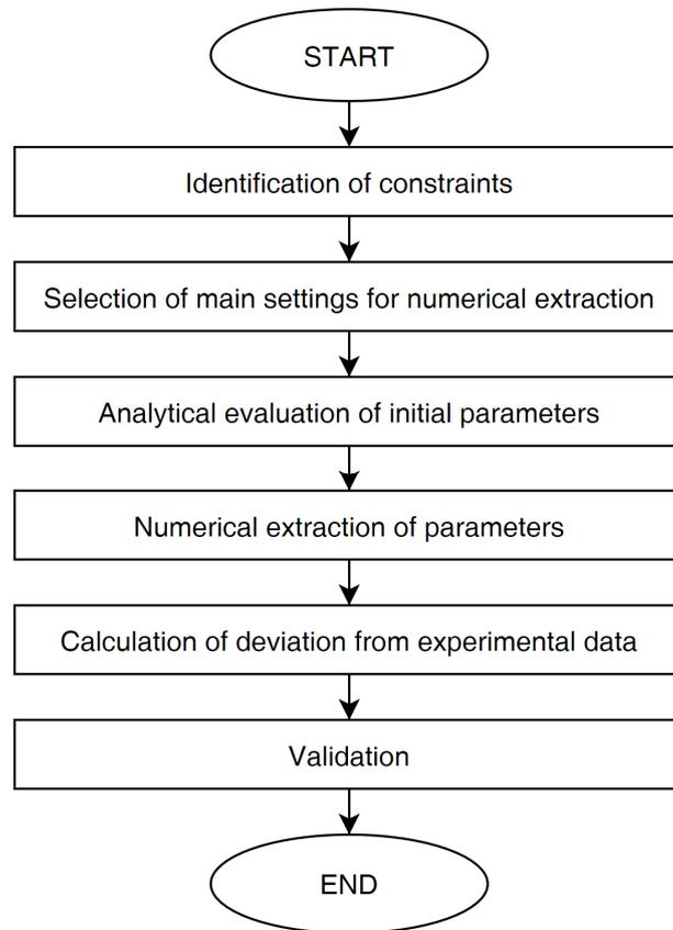
Figure 7.3: Flowchart of the parameters extraction procedure
