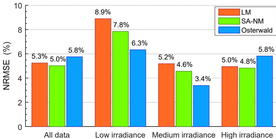
Figure 11.20: *NRMSE* values on estimated power at MPP (division by irradiance)
