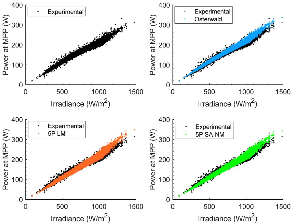
Figure 11.18: Power at different irradiance, experimental value vs the three models (Osterwald in blue, LM in orange, SA-NM in green)
