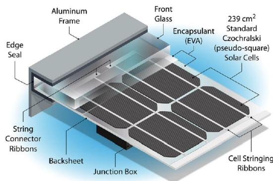
Figure 2.7: Structure details of a photovoltaic module [12]
