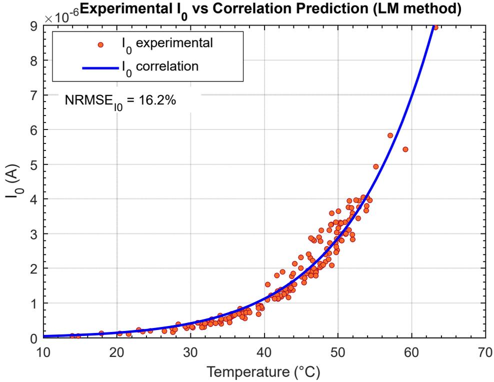
Figure 11.7:  $I_0$  tendency with temperature (LM algorithm)
