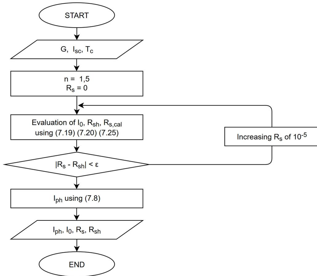
Figure 7.4: Evaluation of initial conditions flow chart
