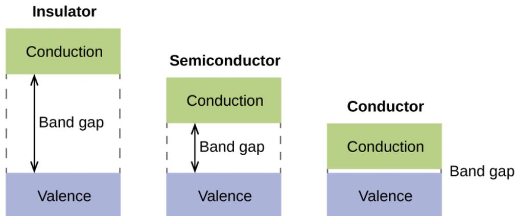
Figure 2.8: Energy gap in different materials [13]
