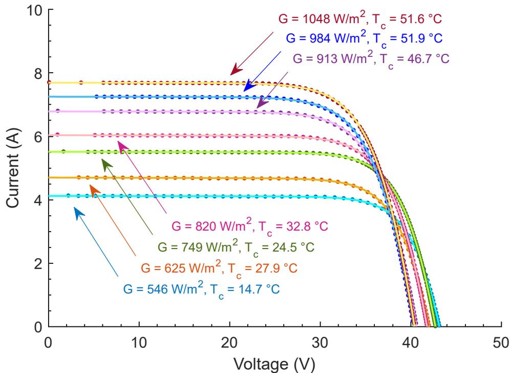
Figure 11.1:  $I$ - $V$  curves experimentally measured (dots) and trend estimated with the LM parameters
