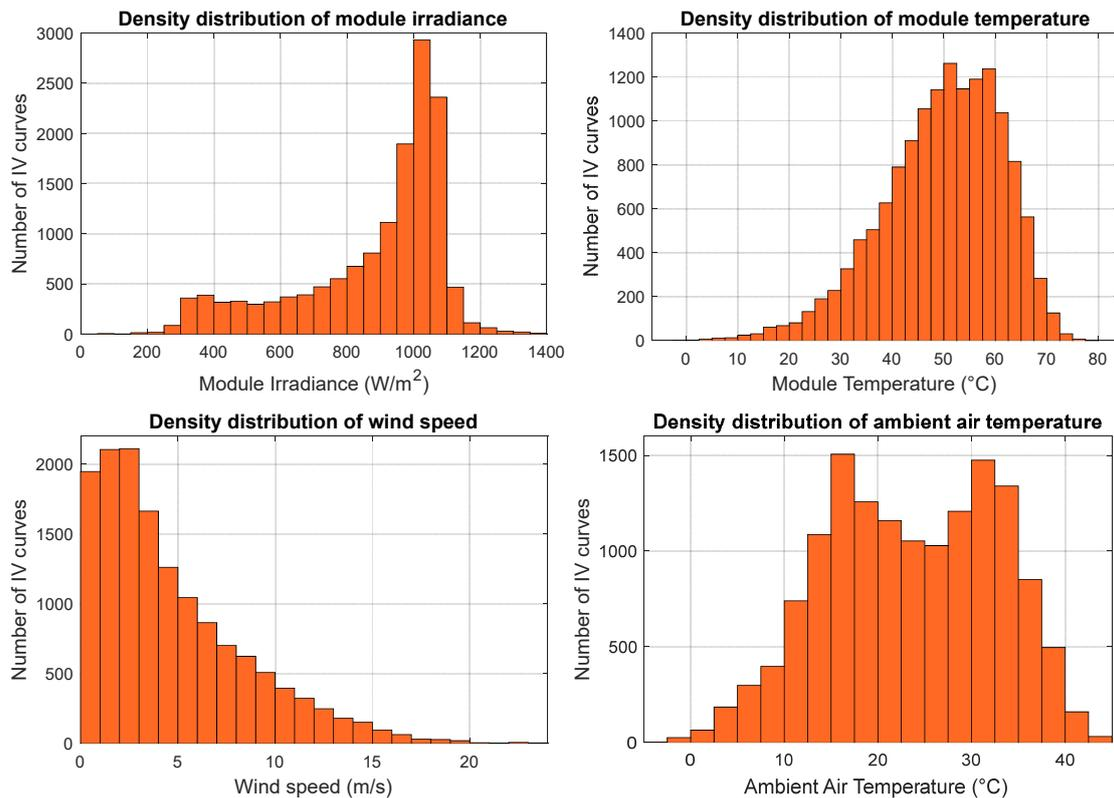
Figure 10.1: Density distribution of the main four environment conditions for HIT module.
