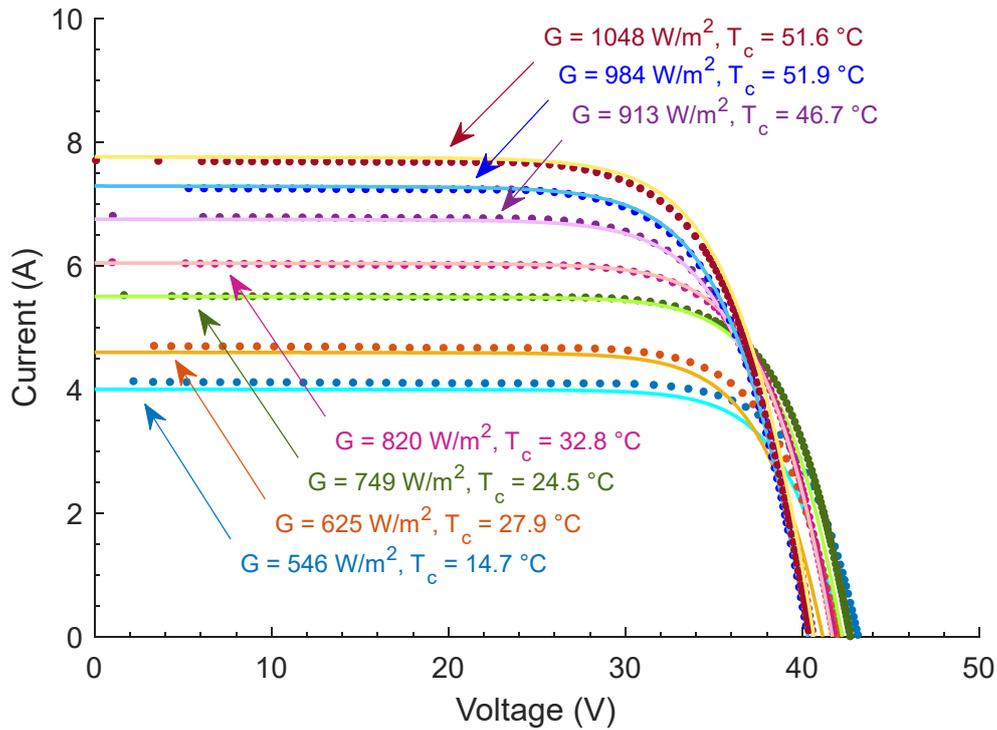
Figure 11.16:  $I$ - $V$  curves experimentally measured (dots) and trend estimated with the correlation (LM method)
