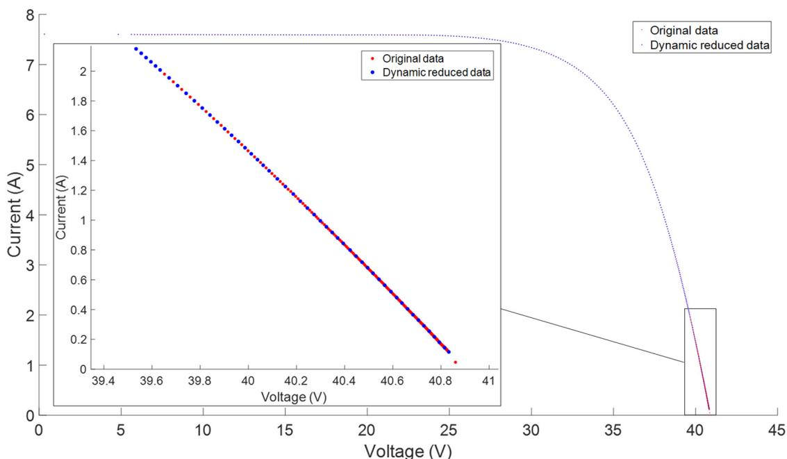
Figure 6.11: Comparison between an original  $I$ - $V$  curve (red) and the dynamic reduced one (blue). The two curves overlap except in the section near the OC point.
