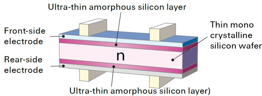
Figure 2.4: Detail of a HIT cell's layer [9]
