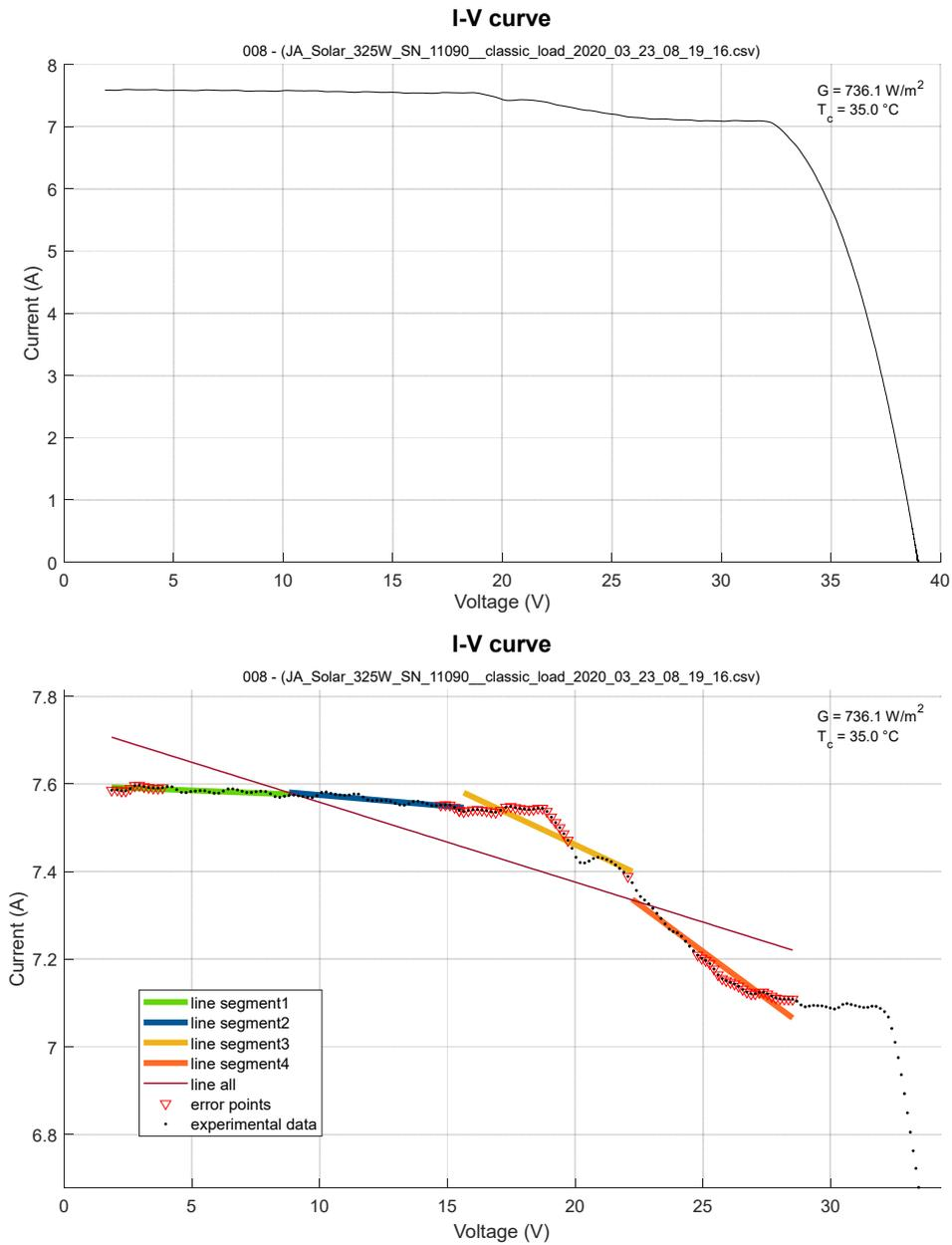
Figure 6.15: Working principles of the mismatch filter on the *I-V* curve.
