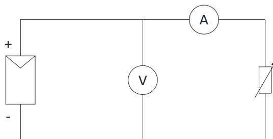
Figure 4.1: Basic schematic of  $I$ - $V$  curve measurement system
