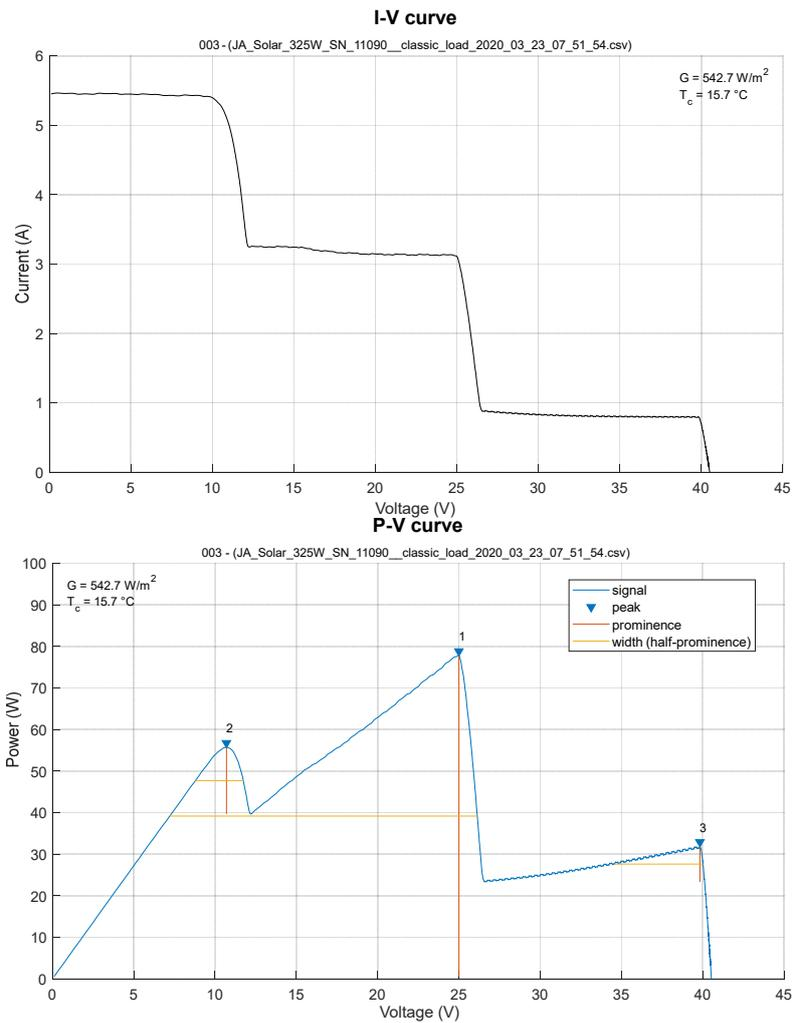
Figure 6.14: Sample of a measure with mismatch.
