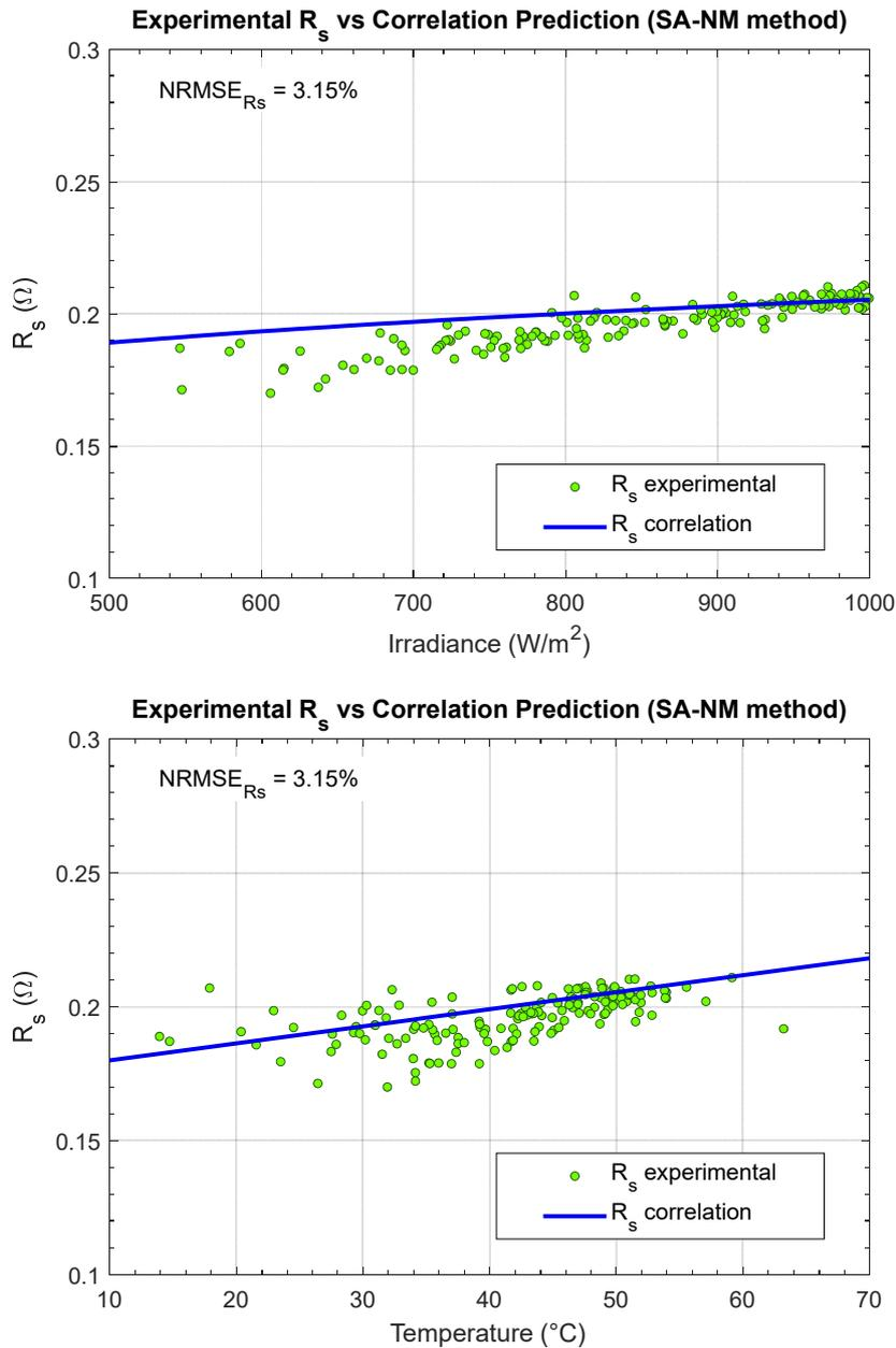
Figure 11.12:  $R_s$  tendency with irradiance and temperature (SA-NM method)
