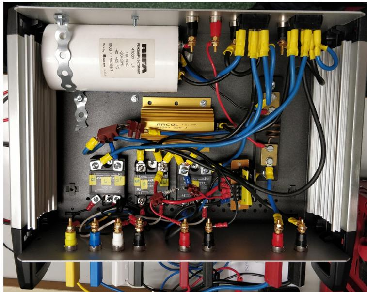
Figure 4.19: View of the inside of the capacitive load
