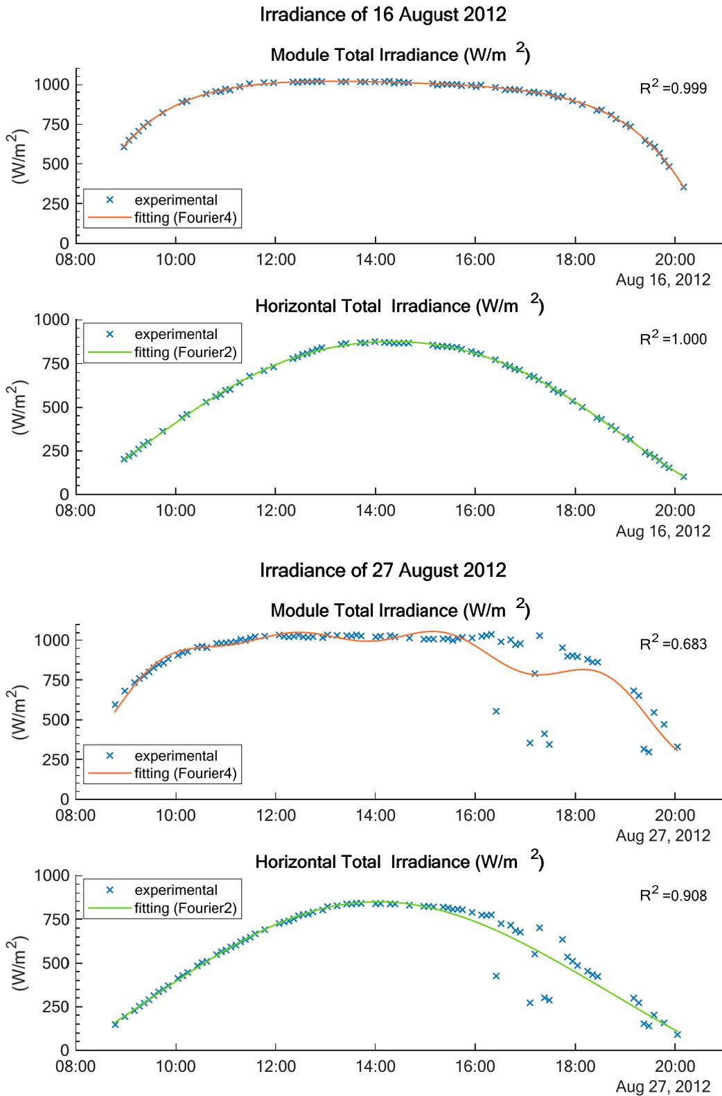
Figure 6.13: Sunny days filter: analysis for two different days. Sunny day upper and non-sunny day lower
