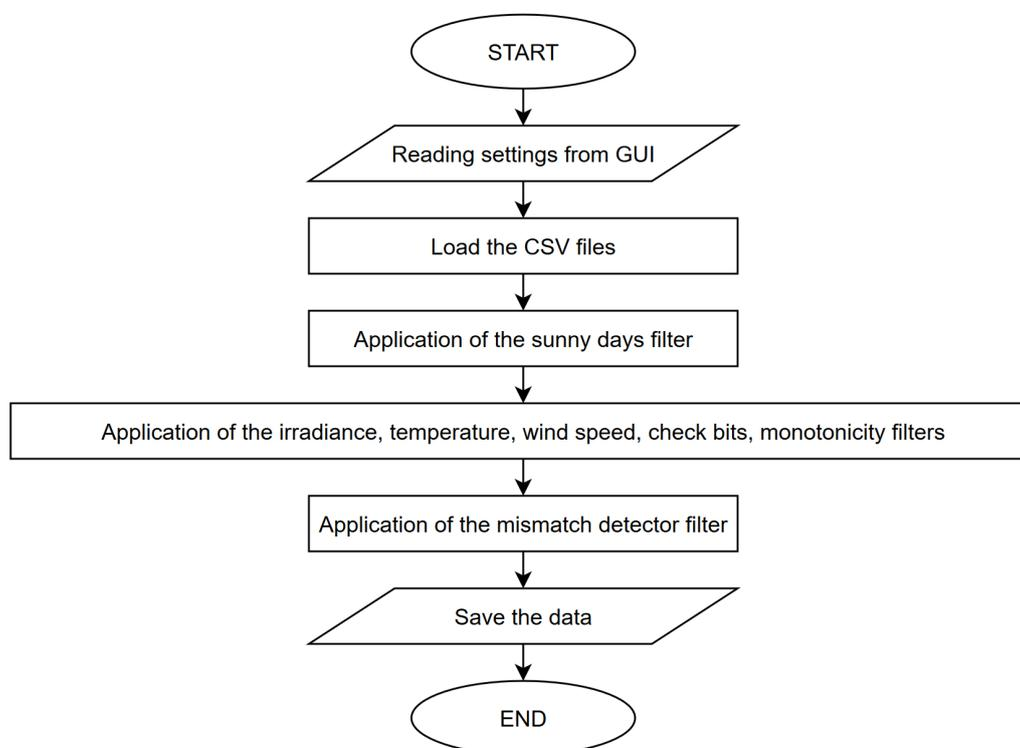
Figure 6.8: Flowchart of the data preprocessing
