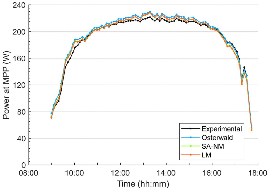
Figure 11.17: Comparison of power estimation for one day.
