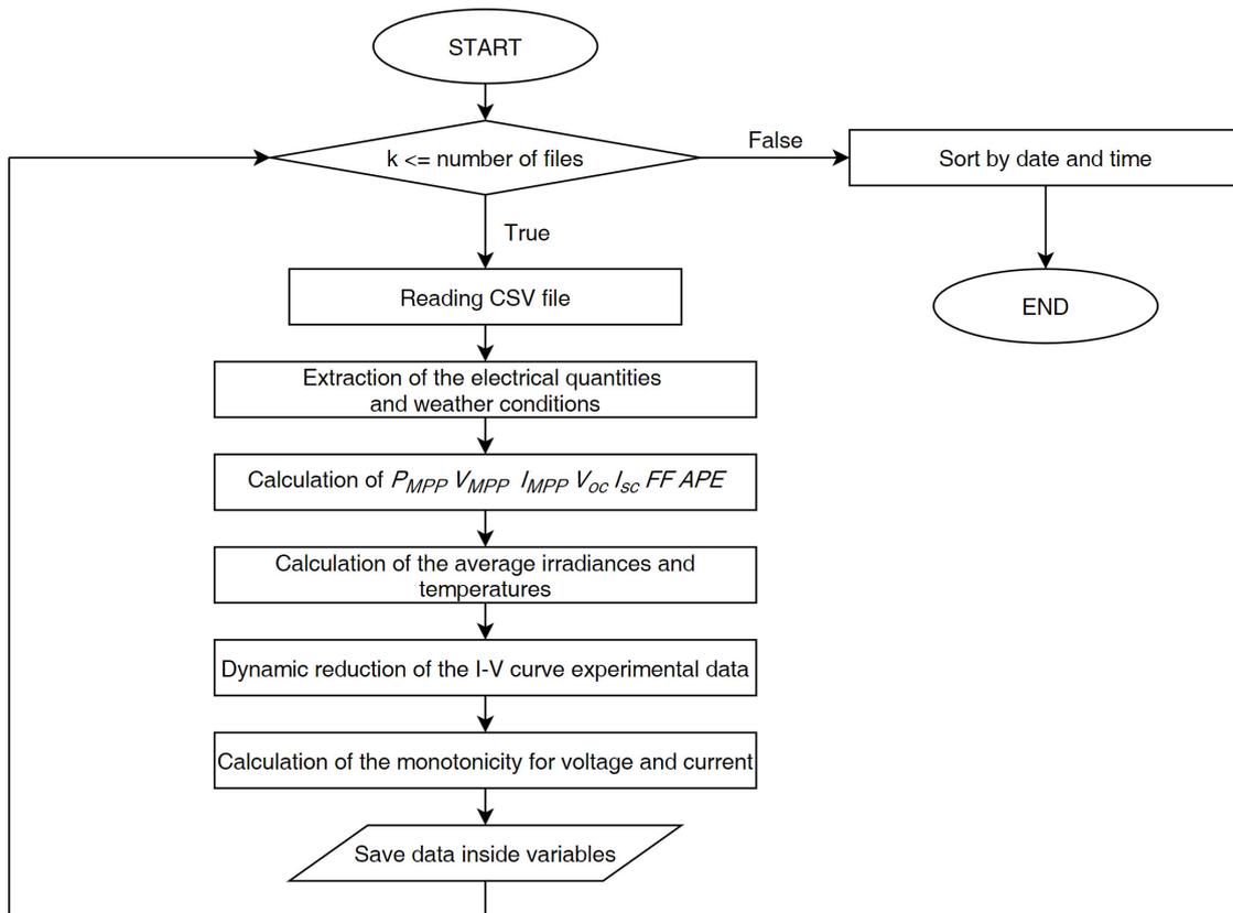
Figure 6.9: Flowchart of the loading process
