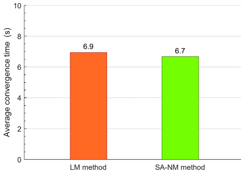
Figure 11.4: Average time to extract the five parameters
