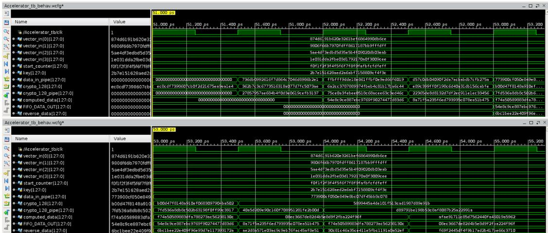
Figure 3.45: Verilog Test-bench - AES-128 Decryption
