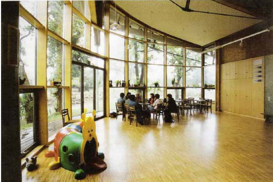
Kindergarten Trinitatis in Riesa, Germany. Sight of the atrium with floor in wood treated with base varnish of soap shellac, non-toxic and easily washable
