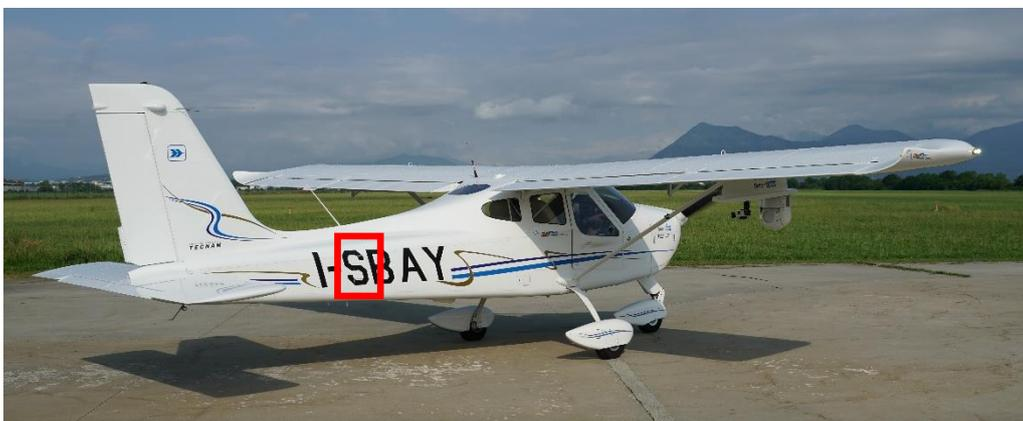
Figure 3-6: Battery compartment location
