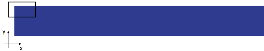
(a) Pristine bondline. The black rectangle frames one of the most critical areas for damage initiation, which is exploited to illustrate fatigue crack growth rate distribution.
