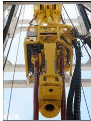
Figure 12: The Top Drive System
