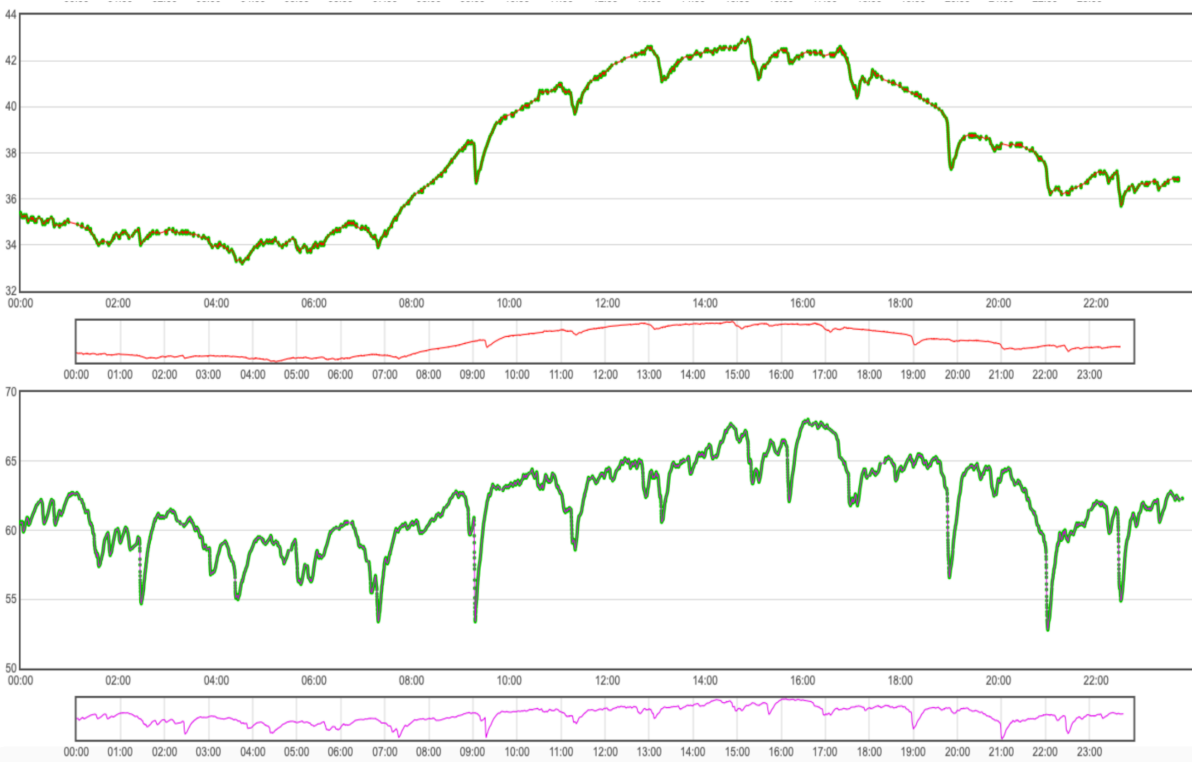
Figure 2.16 Suction and Discharge Temperature Variation of an MPP
