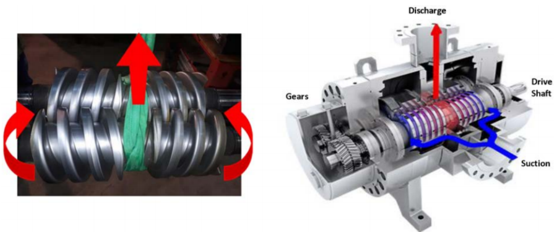
Figure 1.2 Twin screw pump cutaway and flow paths through a rotor assembly
