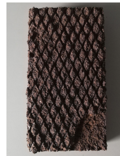
Fig. 73 - Sample C2, 70% coffee grounds and 30% maltodextrin, top view.
