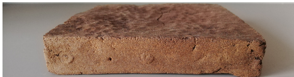
Fig. 72 - Sample C1, 70% coffee grounds and 30% potatoes starch, side view.
