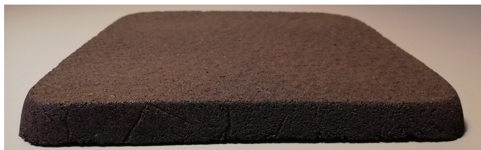
Fig. 78 - Sample C5, 70% coffee grounds and 30% maltodextrin, front view
