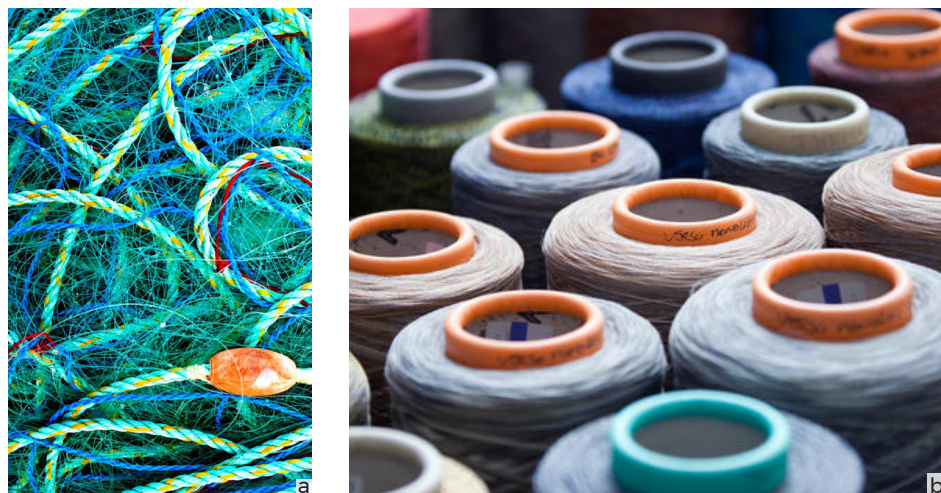
Fig. 4 - Econyl, from fishing net (a) to new yarn (b) by Aquafil (a) https://www.livingcircular.veolia.com/en/industry/econyl-infinitely-recyclable-nylon-yarn (b) https://professionals.tarkett.com/en_EU/node/econyl-recycled-yarn-5248
