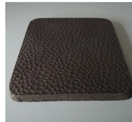
Fig. 79 - Sample D1, 70% coffee grounds and 30% maltodextrin with the bee wax coating
