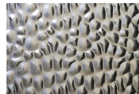
Fig. 70a - Coffee beans texture's mould
