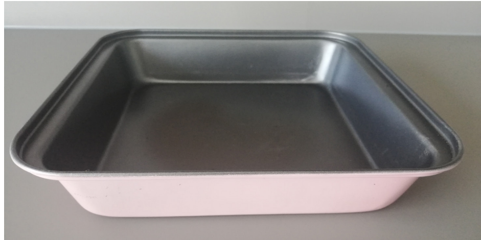
Fig. 55 - Mould 23x23cm, used to produce tiles
