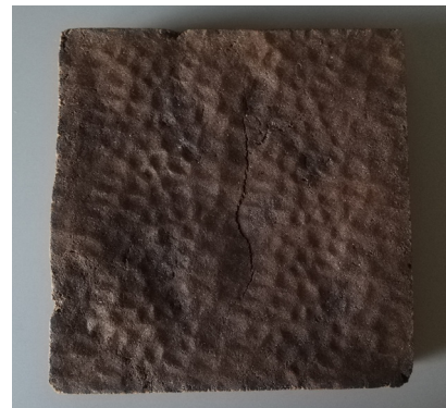
Fig. 71 - Sample C1, 70% coffee grounds and 30% potatoes starch, top view.
