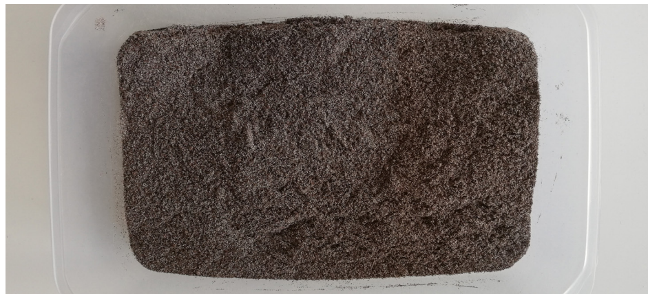
Fig. 50 - Dry homogeneous mixture of spent coffee grounds and dextrin
