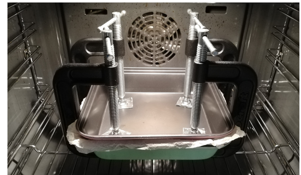
Fig. 58 - Samples have been fired with clamps to maintain the material pressed
