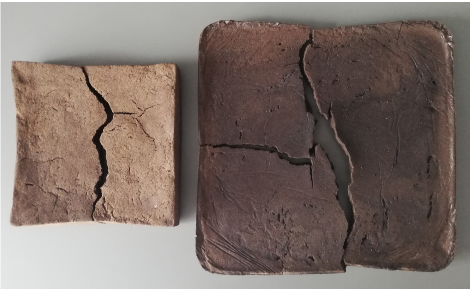
Fig. 83 - Rifts caused by the retrogradation process of the potatoes starch
