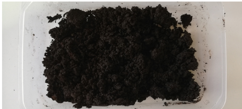
Fig. 51 - Wet homogeneous mixture of spent coffee grounds and dextrin
