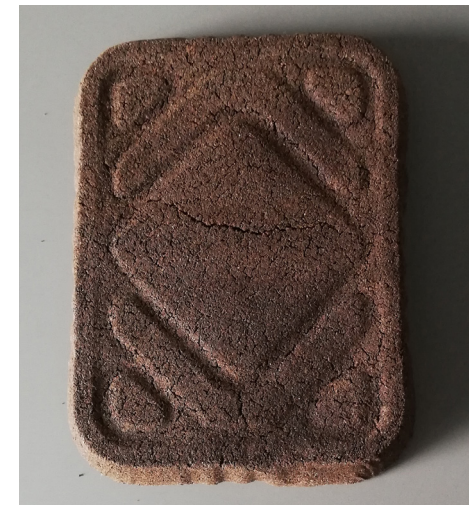
Fig. 65 - Sample A3, 80% coffee grounds and 20% potatoes starch
