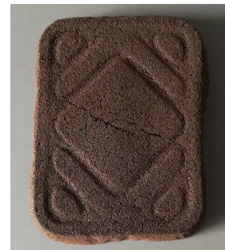
Fig. 66 - Sample A4, 90% coffee grounds and 10% potatoes starch
