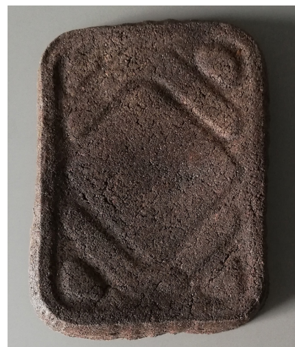
Fig. 63 - Sample A1, 70% coffee grounds and 30% potatoes starch
