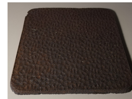
Fig. 80 - Sample D2, 70% coffee grounds and 30% maltodextrin, 1cm thick with the bee wax coating
