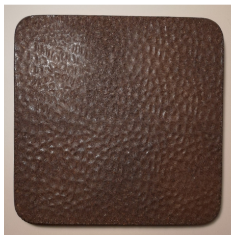
Fig. 77 - Sample C5, 70% coffee grounds and 30% maltodextrin, top view
