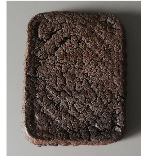
Fig. 64 - Sample A2, 70% coffee grounds and 30% corn starch
