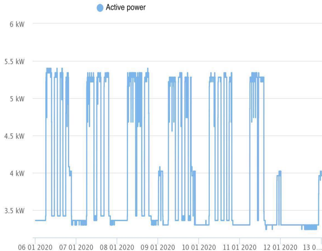
Figure 32 - Weekly active power absorbed by the AHU before the action
