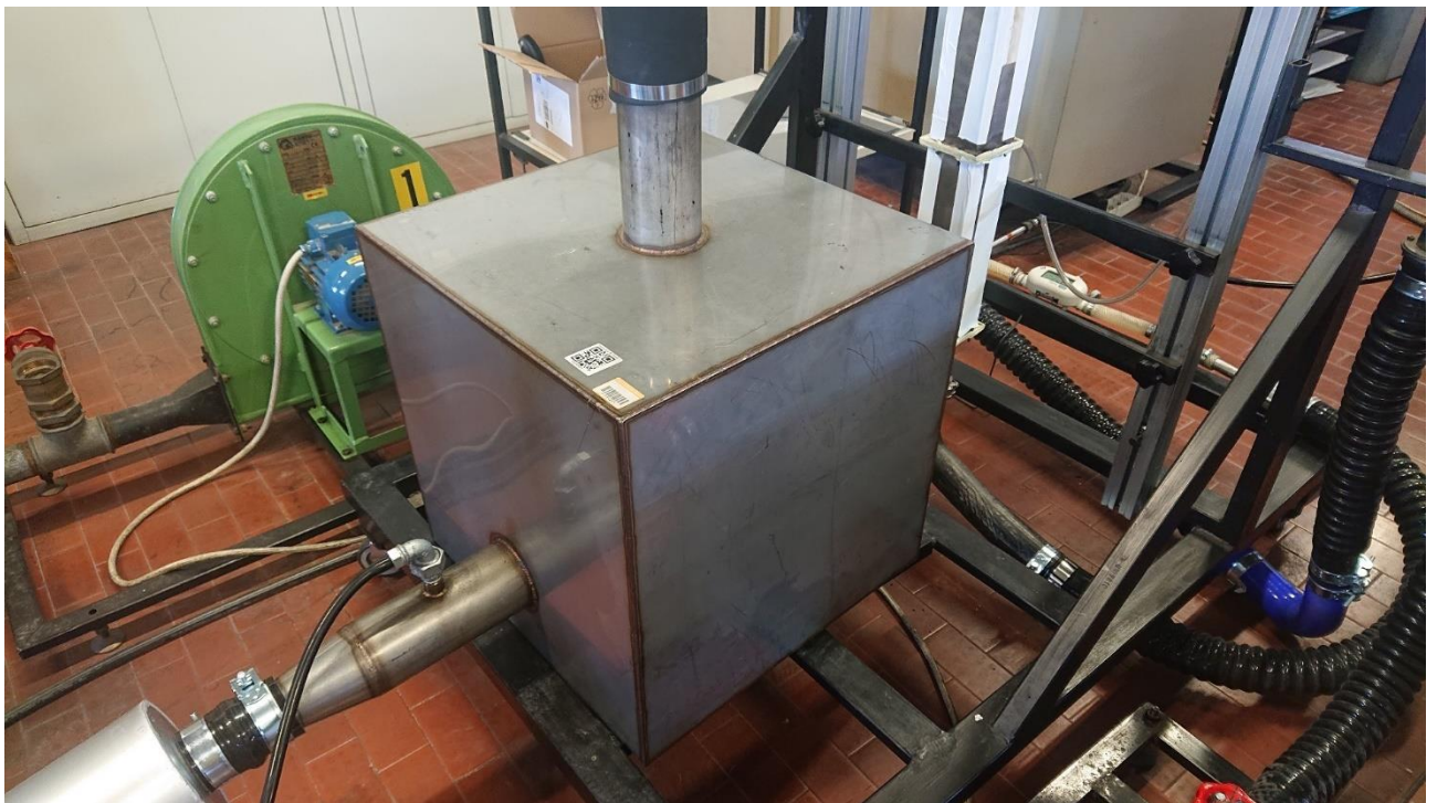
Figure 27. The plenum of the test rig.
