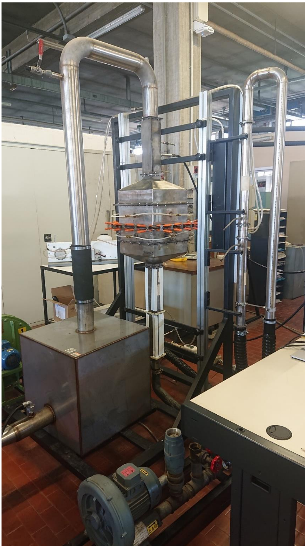
Figure 25. Test rig used to perform fractional efficiency tests
