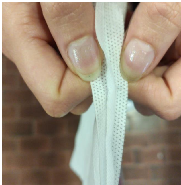
Figure 7. Surgical mask made up of three layers of material (the two external ones of spunbond material and the inner one of meltblown material).
