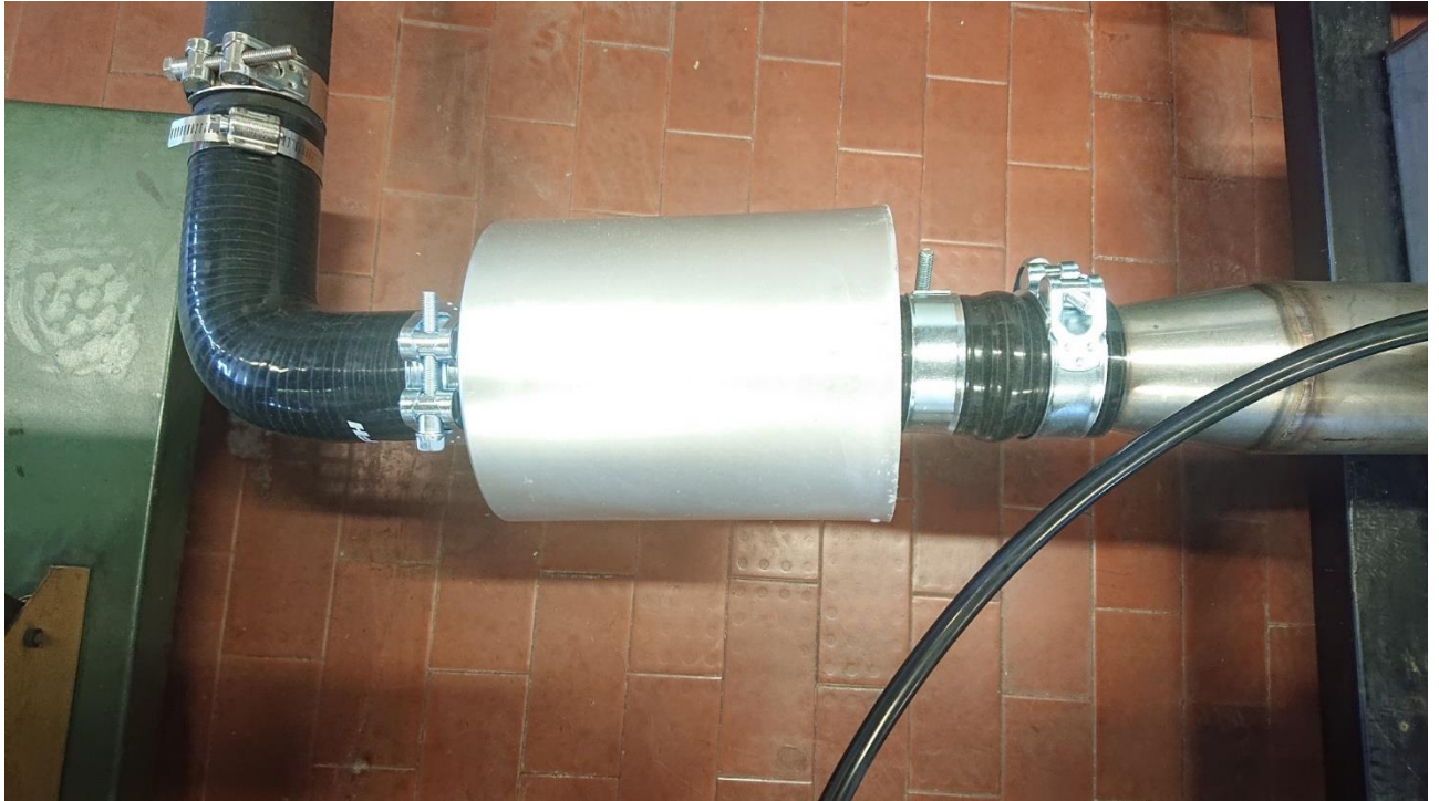
Figure 26. HEPA filter placed just downstream of the upstream fan.
