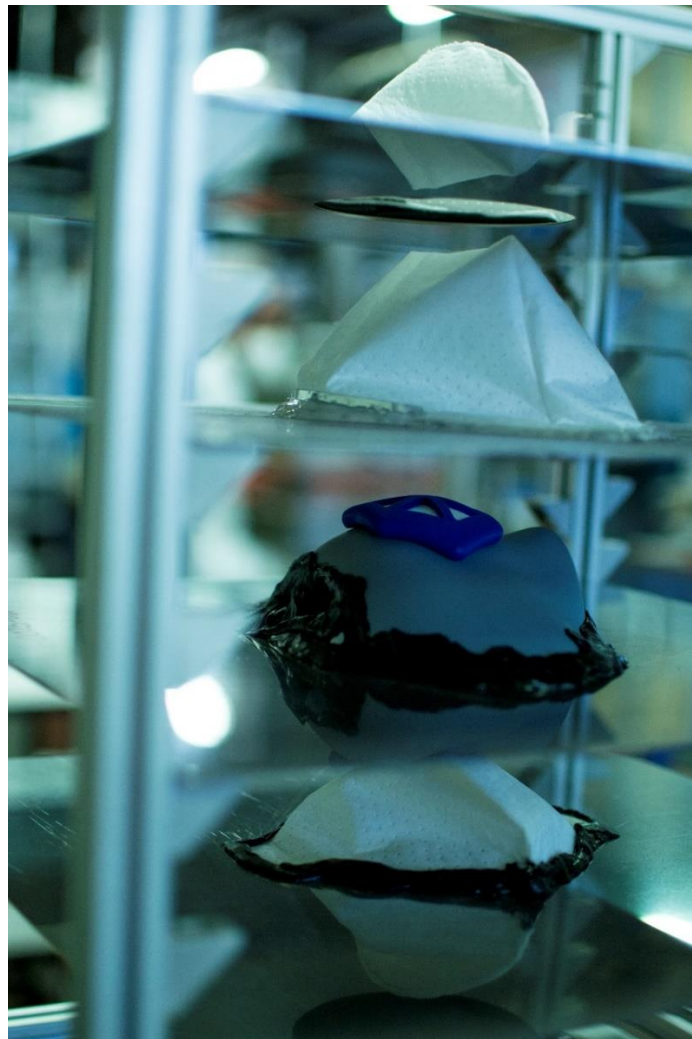
Figure 38. Respirators samples fixed to adapter plates.
