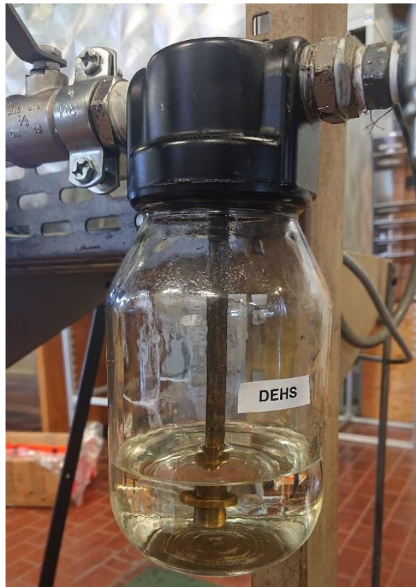
Figure 30. DEHS aerosol generator of the test rig.
