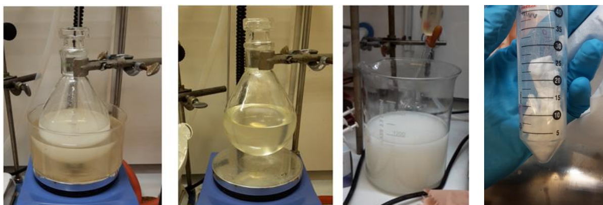
Figure 3.3: Main steps of the starch methacrylation reaction. From the left: starch dissolution in DMSO (a), MA-starch reaction end (b), MA-starch precipitation (c), lyophilized product (d)
