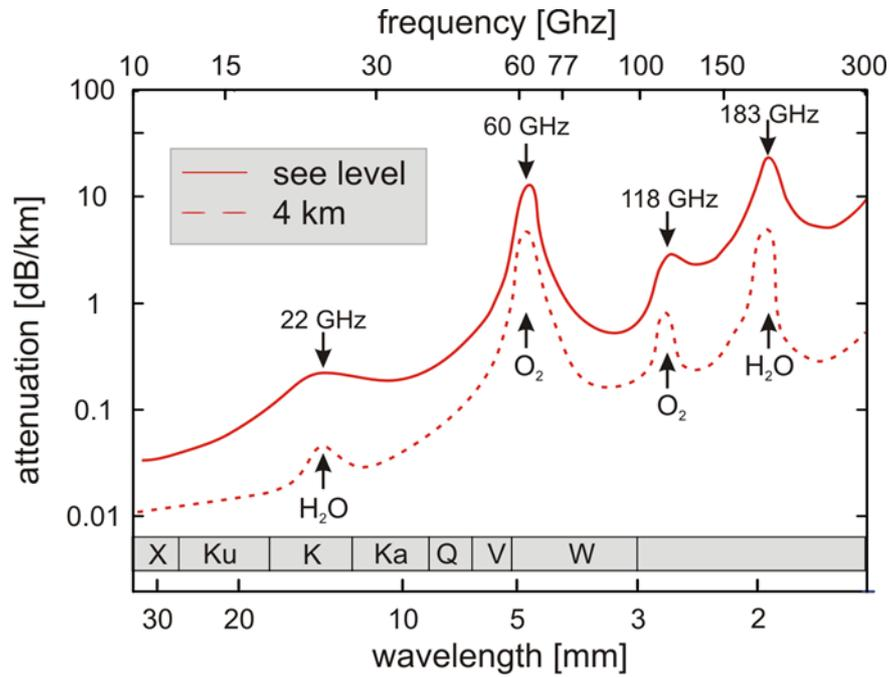
*Figure 8 Atmospheric absorption curve.*
