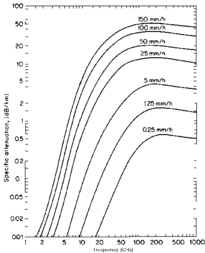
*Figure 9. Specific attenuation for different frequencies and rain rates*
