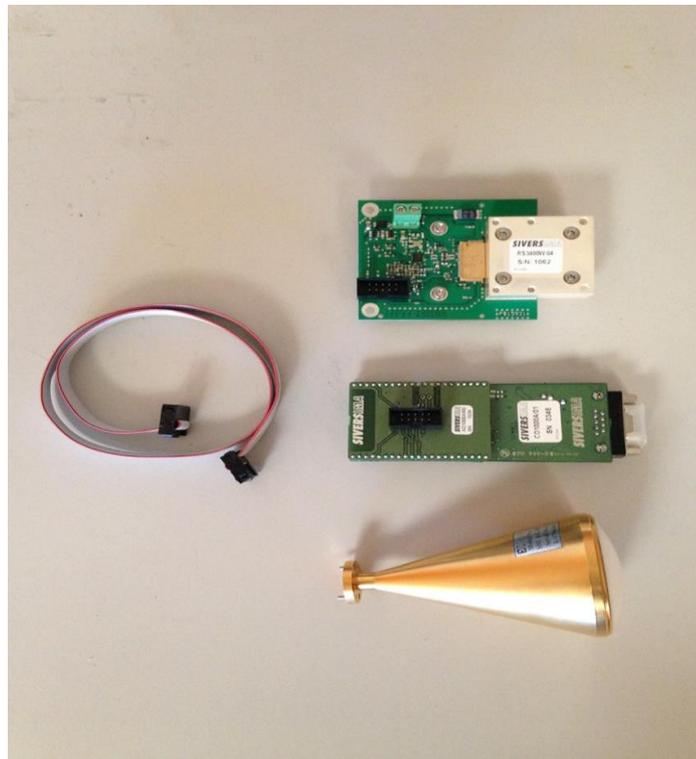
*Figure 10. Radar sensor and antenna*
