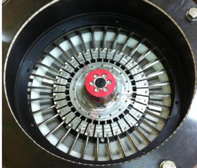
Figure 6.3: The dummy disk 2 within the spinning test rig [3]
