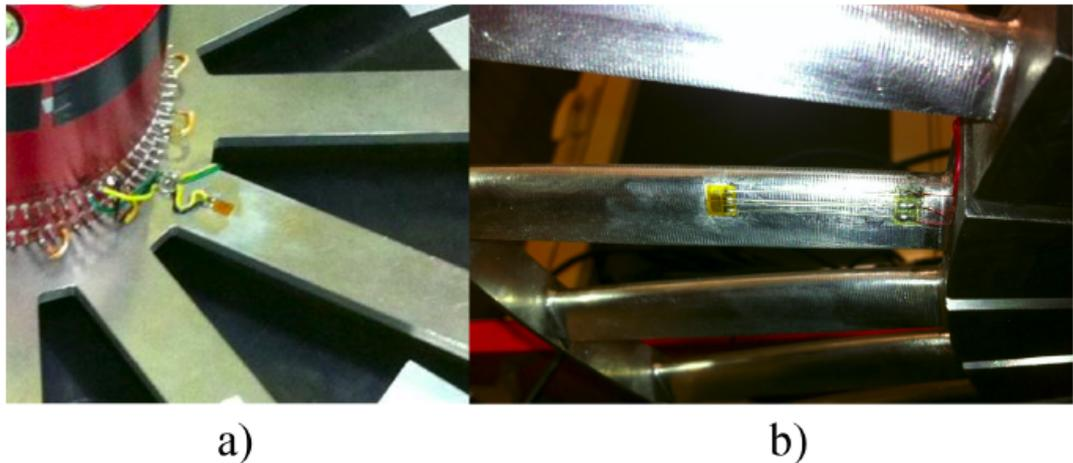
Figure 6.7: Strain gauge at the blade root of the dummy disk 1 a), strain gauge at the back of the airfoil of a dummy disk 2 blade b) [3]
