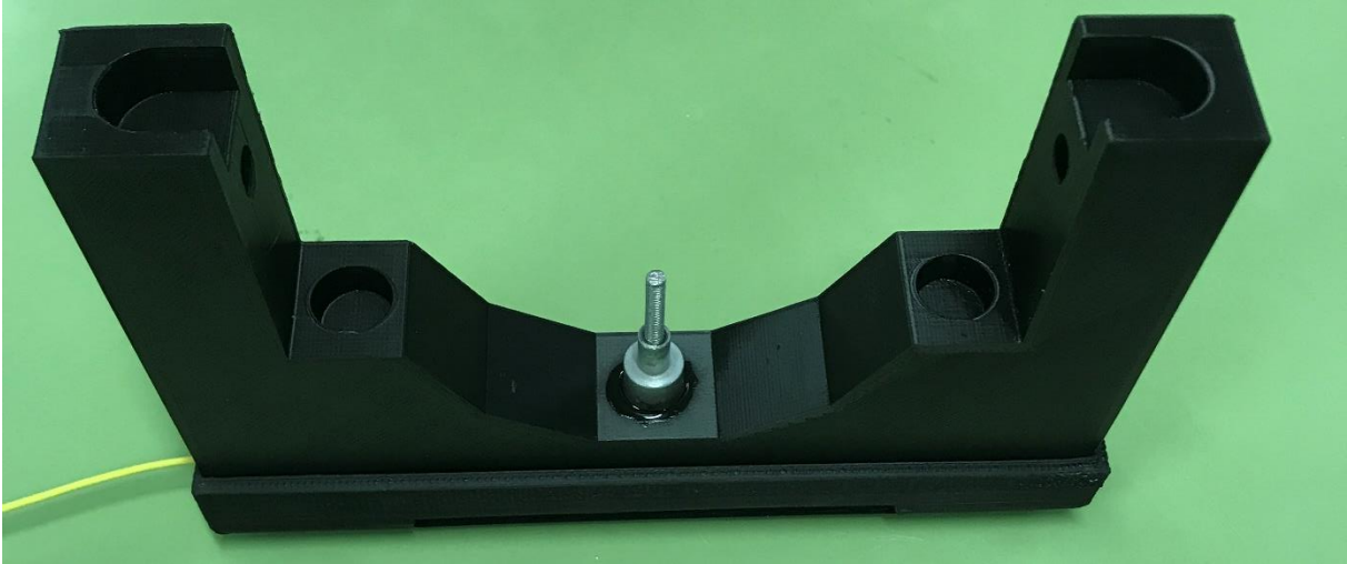
FIGURE 52: THE FBG SUPPORT MODIFIED
