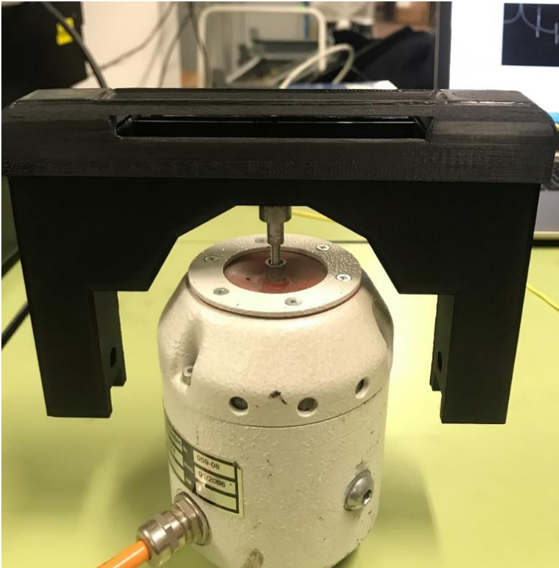
FIGURE 53: FBG SUPPORT MOUNTED ON THE SHAKER
