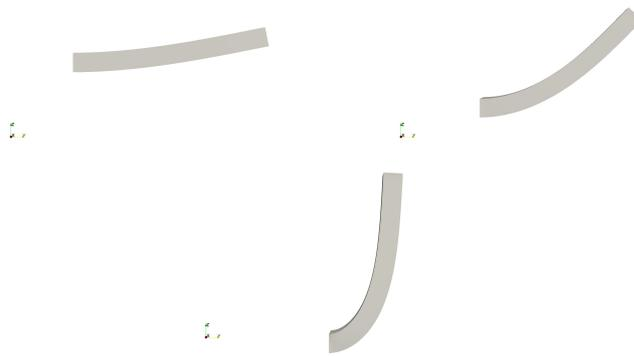
Figure 3.2: Deformed shape for three different load values - square beam
