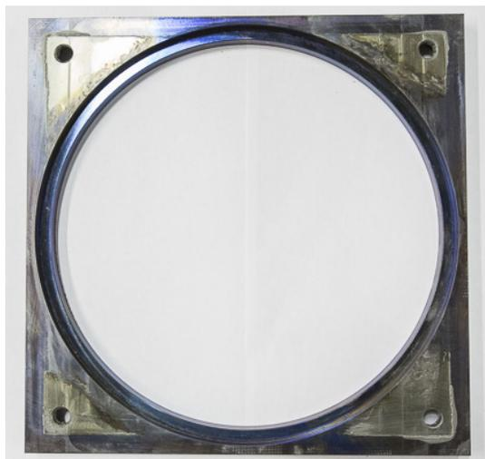
**Figure 4.7:** Clamping plate
