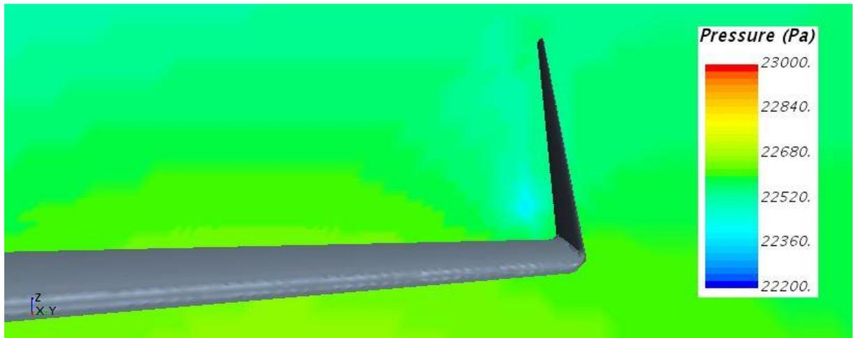
Figure 54 – Blended winglet pressure field behind wing
