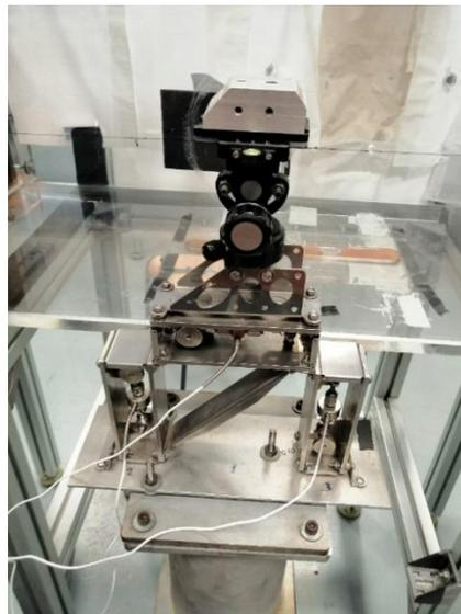
Figure 19 - Balance with gauges
