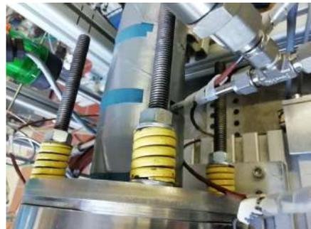
(b) Detail of springs holding the combustion chamber.
