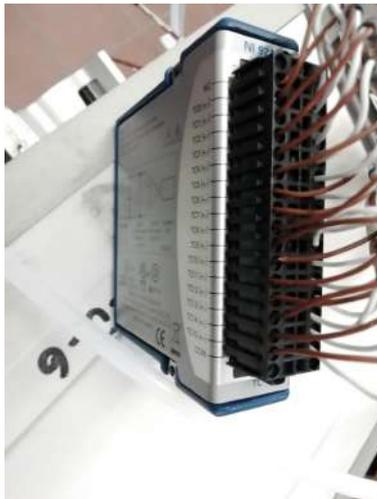
(a) Thermocouples inserted into the cart module.
