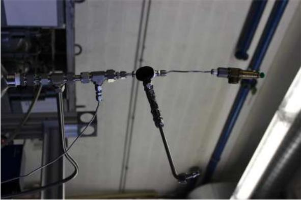
(e) Over pressure valve - Check valve - Release valve.
