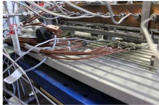
(b) Combustion chamber thermocouples.
