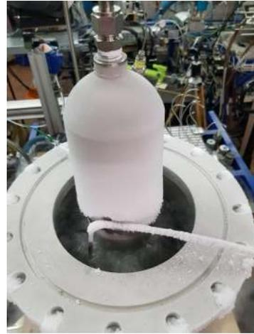
(b) Liquifier filled with liquid nitrogen.
