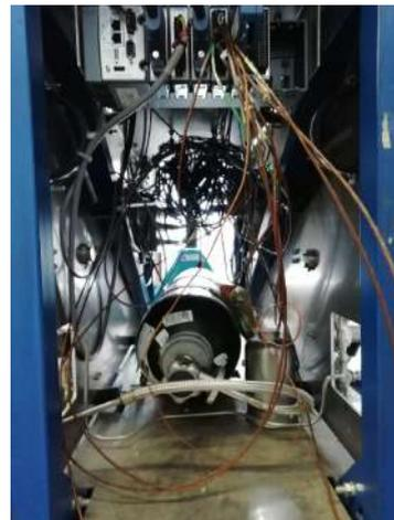
(b) Cart module inserted into MoRap.
