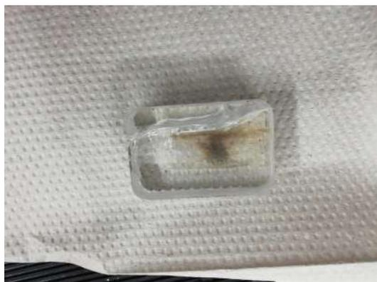
(b) Window breaking after Hot Fire test.
