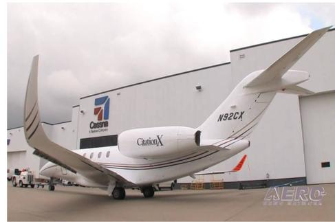
Figura 1.7: Elliptical Winglet, [31]
