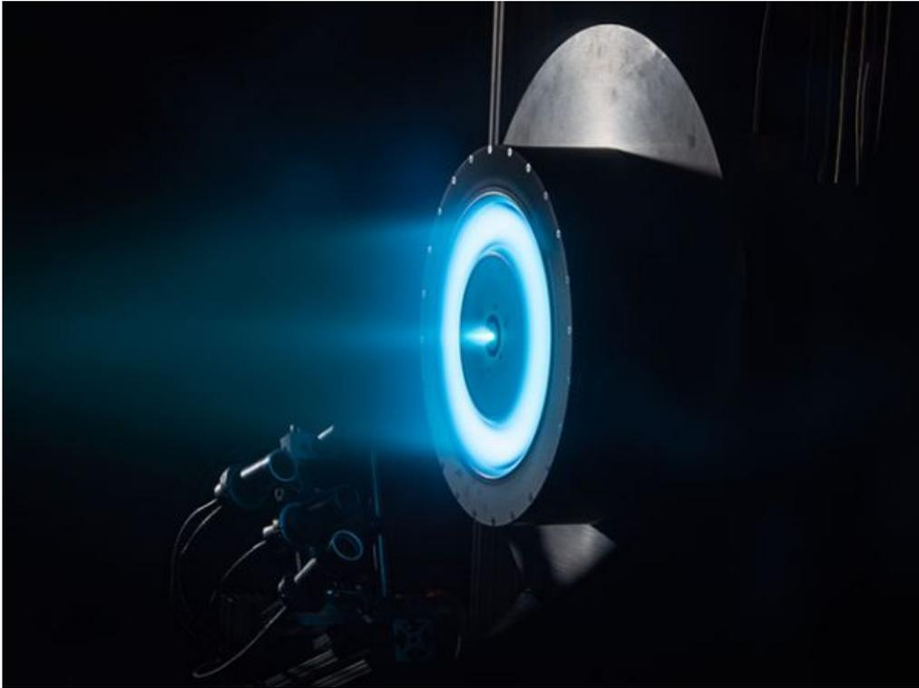
Figure 4.8: Blue ion beam of a Hall Thruster
