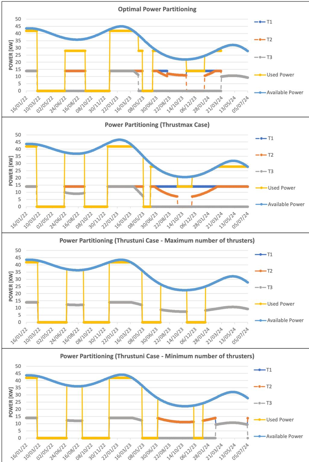
Figure 8.2: Power partitioning between thrusters
