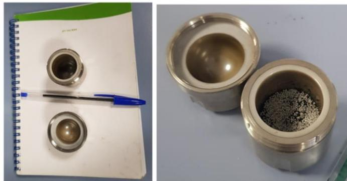
Figure 8- left) comparison of the dimension with a pen; right) chamber refill with zirconia balls and  $\text{Co}_3\text{O}_4$  powder
