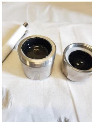
*Figure 10 - Slurry after the Milling process*
