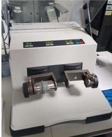
*Figure 9- Milling machine, Retsch MM 400*
