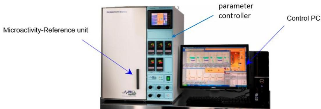
Figure 23 - Main elements of the reactor setup
