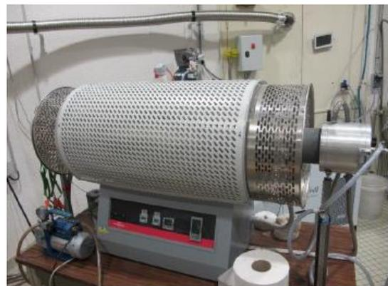
Figure 6 - Oven for debinding (IREC)
