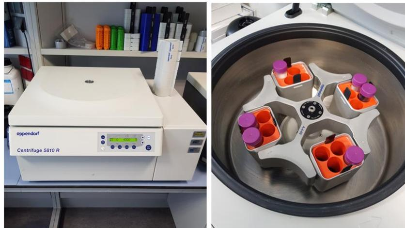
*Figure 11 - Centrifuge machine (Eppendorf 5810 R)*
