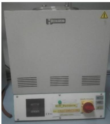
Figure 13- oven for the calcination of the catalyst
