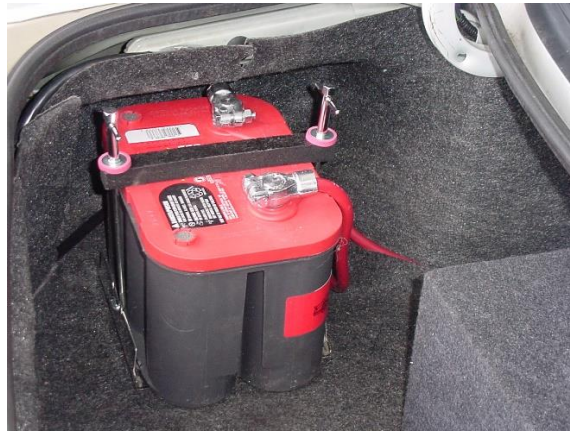
Figure 91. Battery location in the trunk of the car
