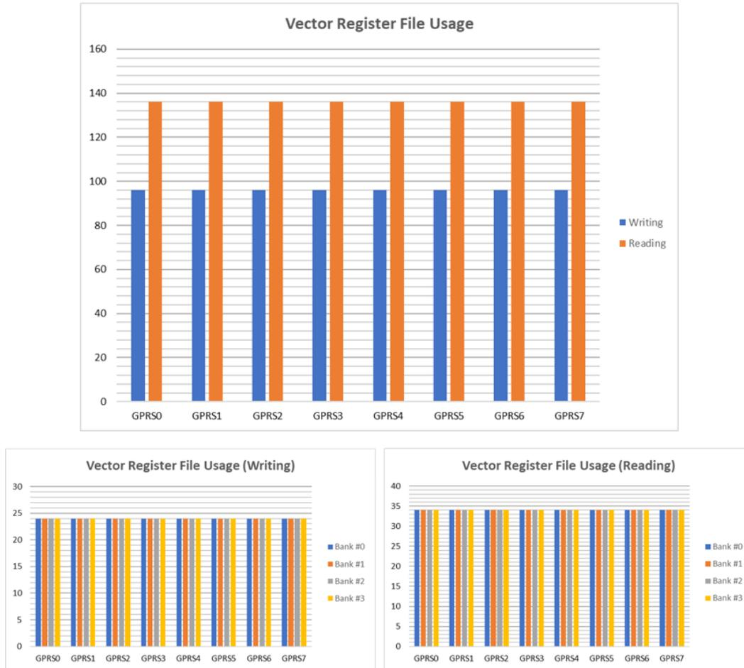
Figure 5.18: Vector\_sum with resilient global access: *vector register file* monitoring results.
