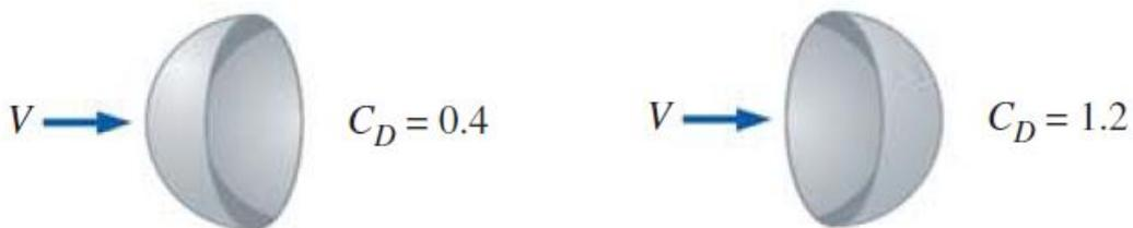
Figure 19 The effect of the shape on the drag coefficient [17].
