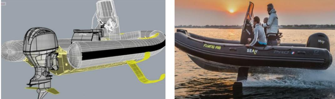
Figure 2 hydrofoil boat, foils create a lift force that can emerge the boat from the water at high velocities
