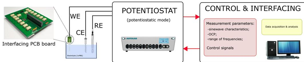
Figure 4.10: Measurement setup for EIS characterization
