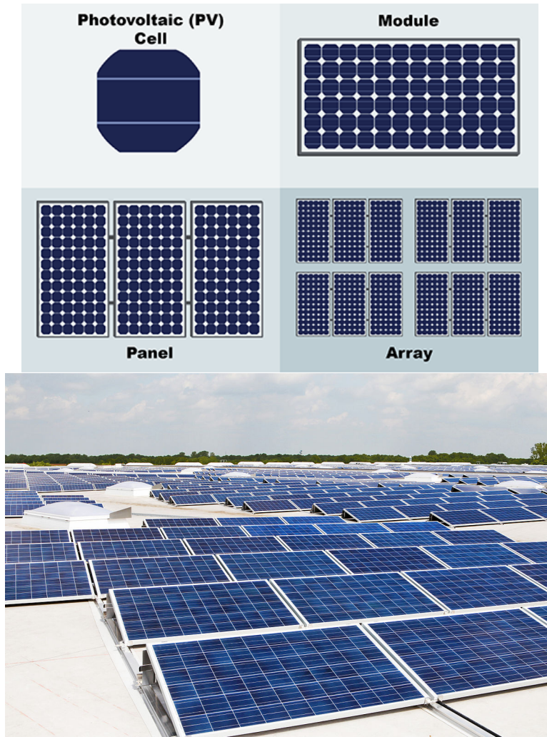
Figure 2.3. Solar cells arrangement (a)-(b) [8]-[9]
