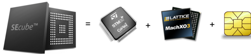
Figure 3.1. The components of the SEcube.
