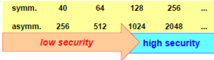
Figure 3.5: Key strength of both symmetric and asymmetric algorithms
