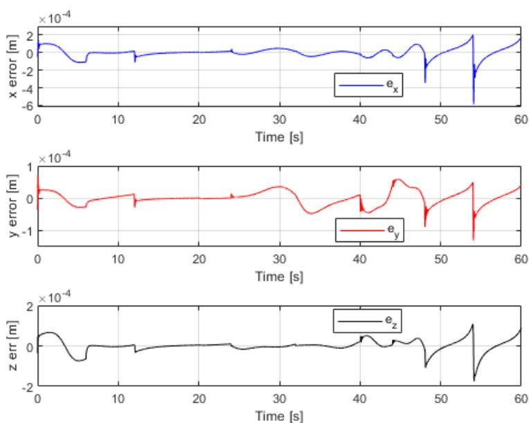
Figure 39: Errors of the end effector position in 3D space
