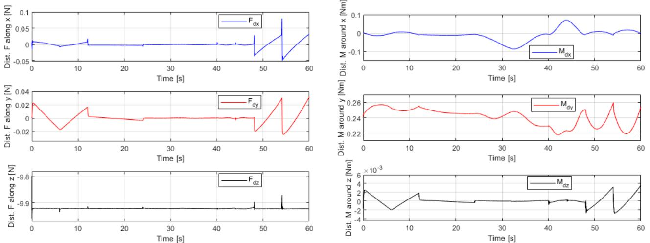
Figure 33: Disturbance forces transmitted from the robot to the hexacopter
