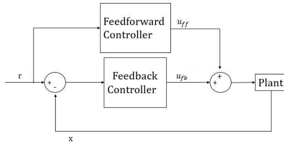
Figure 16: General control architecture based on feedforward and feedback component
