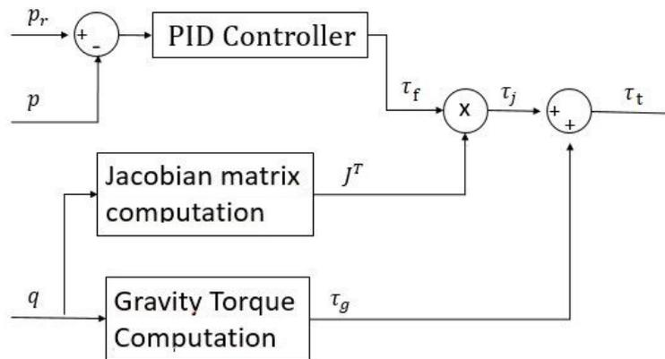
Figure 19: Operational space controller with gravity compensation
