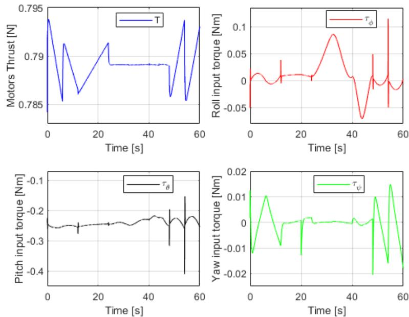
Figure 34: Control inputs to the hexacopter system
