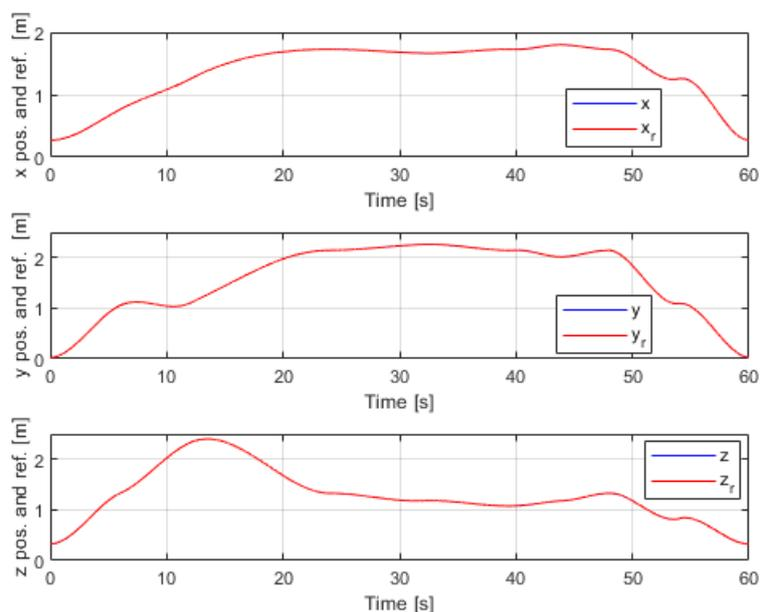
Figure 38: Position values and references of the manipulator
