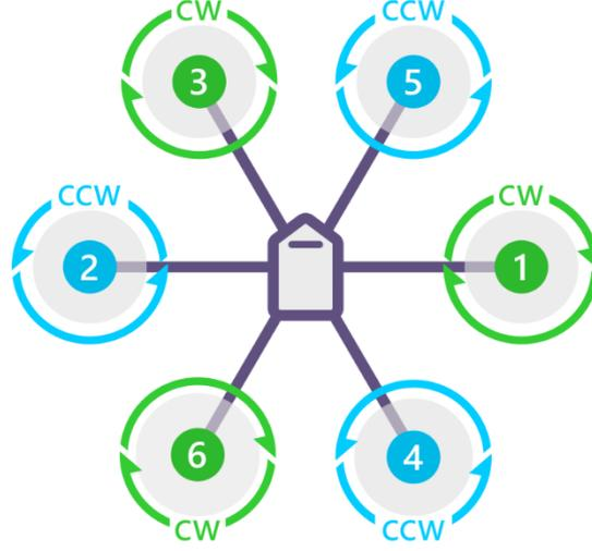
Figure 1: Schematics of hexacopter's motors configuration
