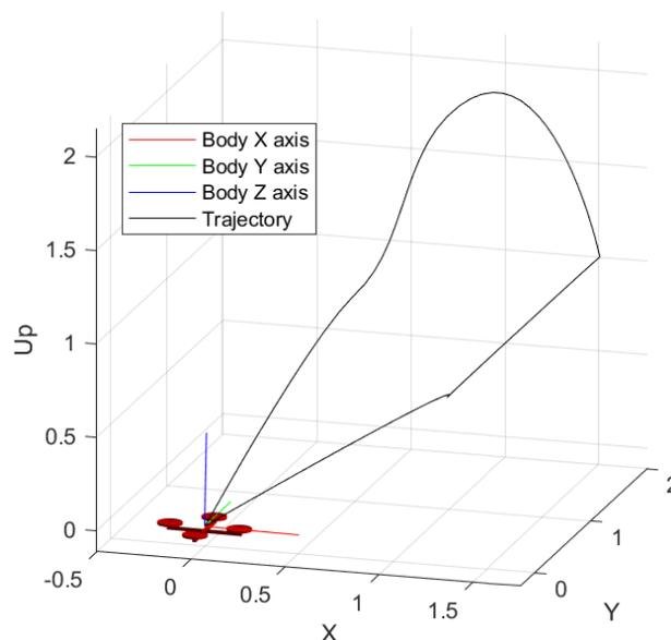
Figure 43: Trajectory followed by the hexacopter during the simulation
