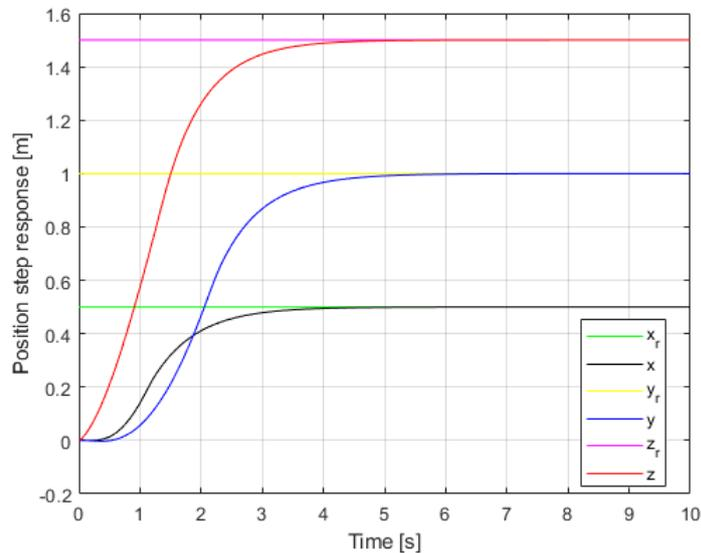
Figure 11: Inertial position step response
