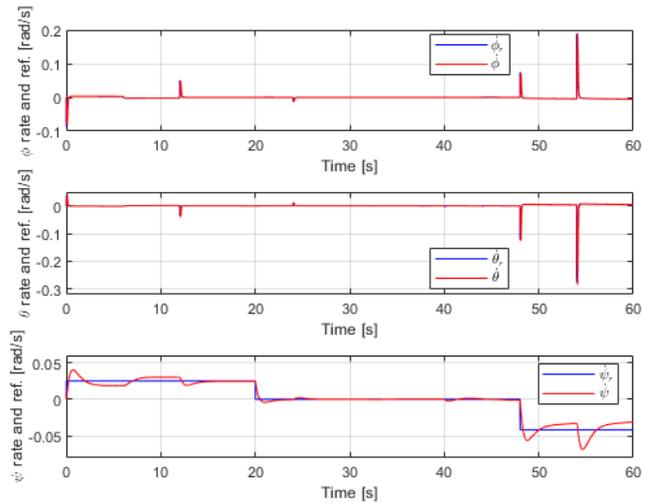
Figure 35: Angular velocity values and references of the hexacopter
