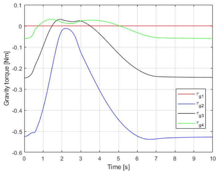
Figure 25: Gravity compensation torque
