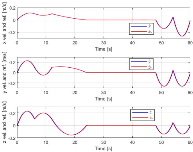
Figure 36: Linear velocity values and references of the hexacopter
