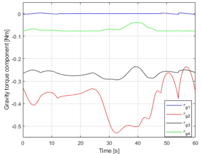
Figure 41: Joints gravity torque components of the control action
