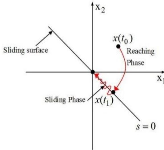
Figure 9: Behaviour of the system under the effect of a sliding mode controller
