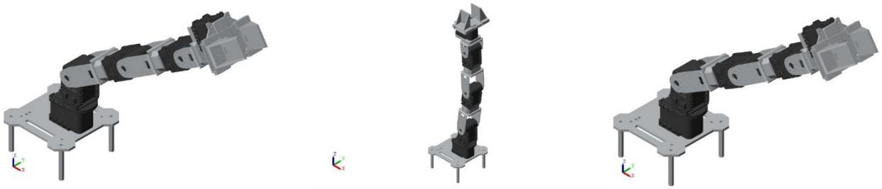
Figure 20: Simscape visualization of manipulator motion
