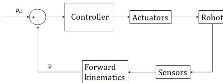
Figure 18: Task space control architecture
