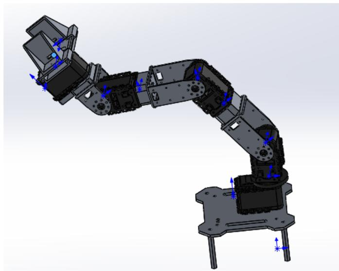
Figure 3: SolidWorks model of the manipulator
