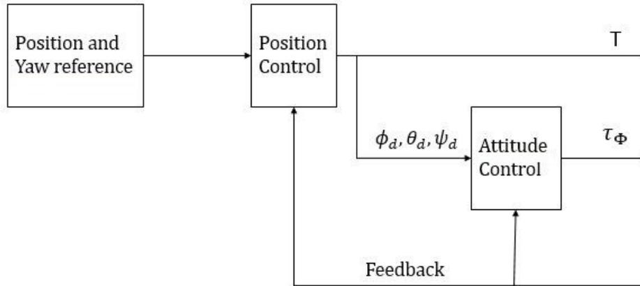
Figure 8: Hierarchical control scheme of the hexacopter
