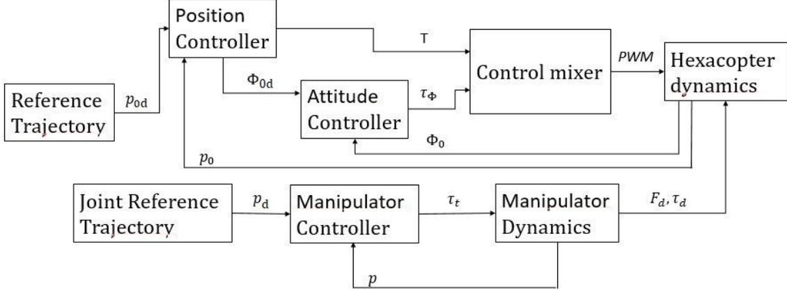
Figure 6: Overall control architecture after coupling the two systems
