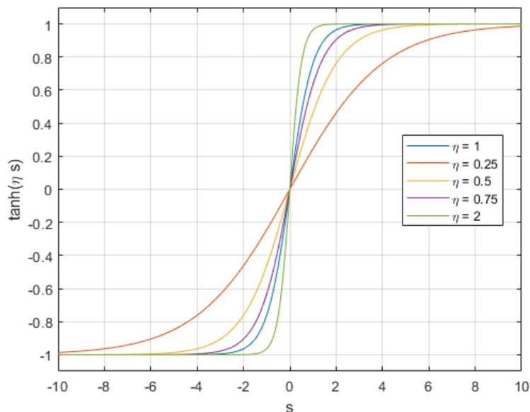
Figure 10: Hyperbolic tangent depending on the  $\eta$  parameter
