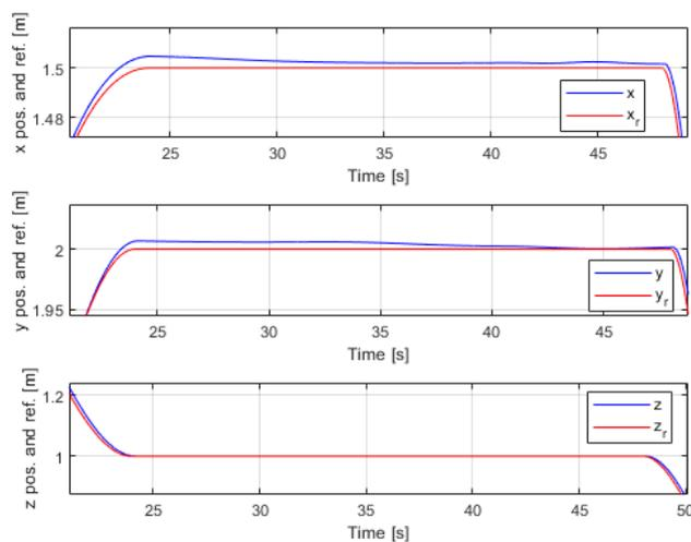
Figure 28: Detail of position values and references of the hexacopter
