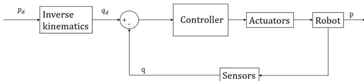
Figure 17: Joint space control architecture
