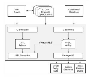
Figure 2.10: Vivado HLS Design Flow
