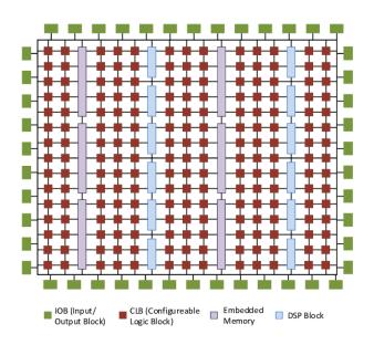
Figure 2.8: Modern Xilinx FPGA Architecture
