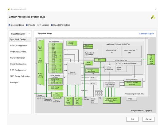
Figure 4.10: The Presetting of ZYNQ7 Processing System
