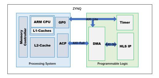
Figure 4.14: Block Diagram of Communicating with DMA
