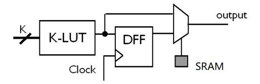
Figure 2.7: The Basic Structure of Logic Elements
