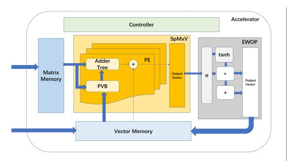
Figure 4.3: Overall Architecture of LSTM accelerator
