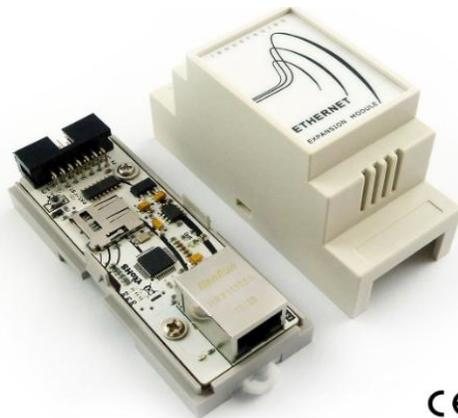
Figure 3.2.4.1 Ethernet expansion module
