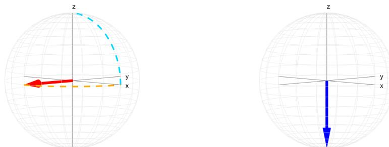
(c) The system evolves for a time  $t = \frac{1}{2J}$ , after which the target qubit lies on the  $-\hat{y}$  axis.
