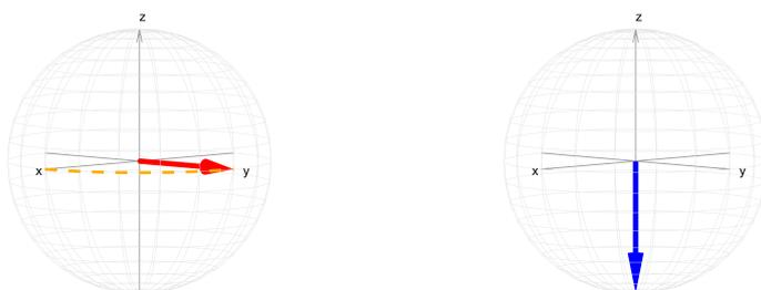
(c) A rotation  $\mathbf{R}_x(\pi)$  is applied to qubit-3 which ends up in the  $|1\rangle$  state.
