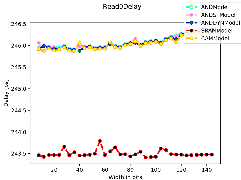
Figure 7.1: Read operation delay: cell content equal to ‘0’, ideal drivers.
