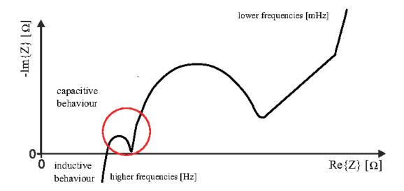
Figure 7 The behaviour of the battery's impedance with different frequencies.
