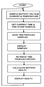
Figure 5 Flow chart of the processes performed by the patented device.
