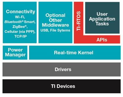
Figure 16. TI RTOS Components Layers
