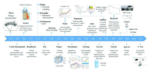
Figure 4 Trials of 'SoH' and 'SoC' estimation from 1938 to 2017.
